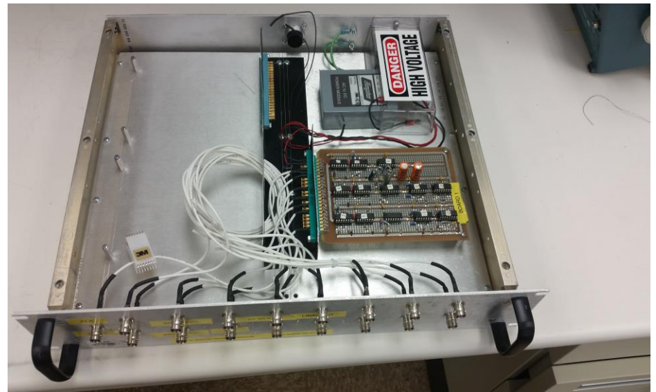
Fig. 4 switching circuit prototype in chassis
