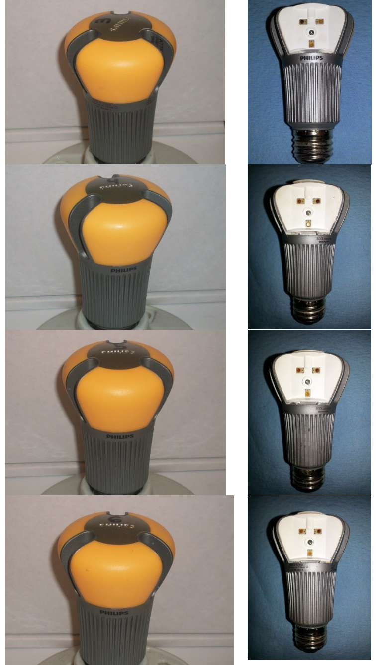
Figure 16 Representative Samples of the Failed Lamps with and without the Lens. Encapsulant of several of the LEDs in the failed lamps shows distinct discoloration
