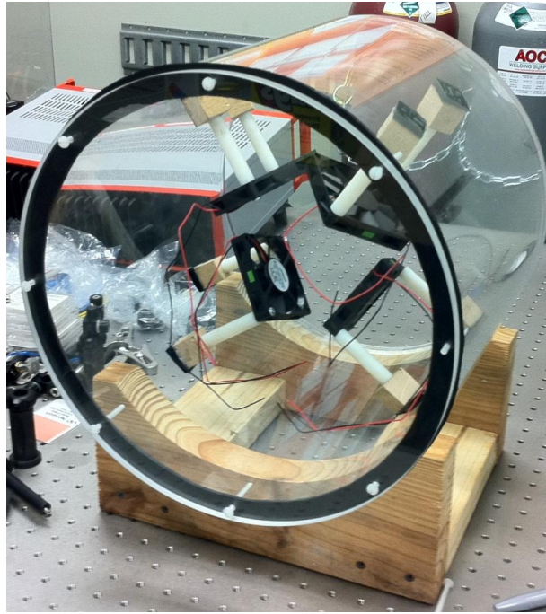
Fig. 2 Photograph of plexiglass mock-up facility showing a trial fan placement.
