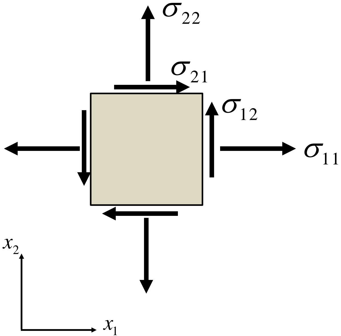
Hooke's Law is like a spring but in all directions and including shear. We use a 4<sup>th</sup> order tensor
