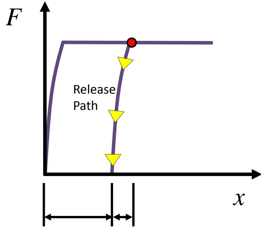
Plastic Deformation      Elastic Deformation
