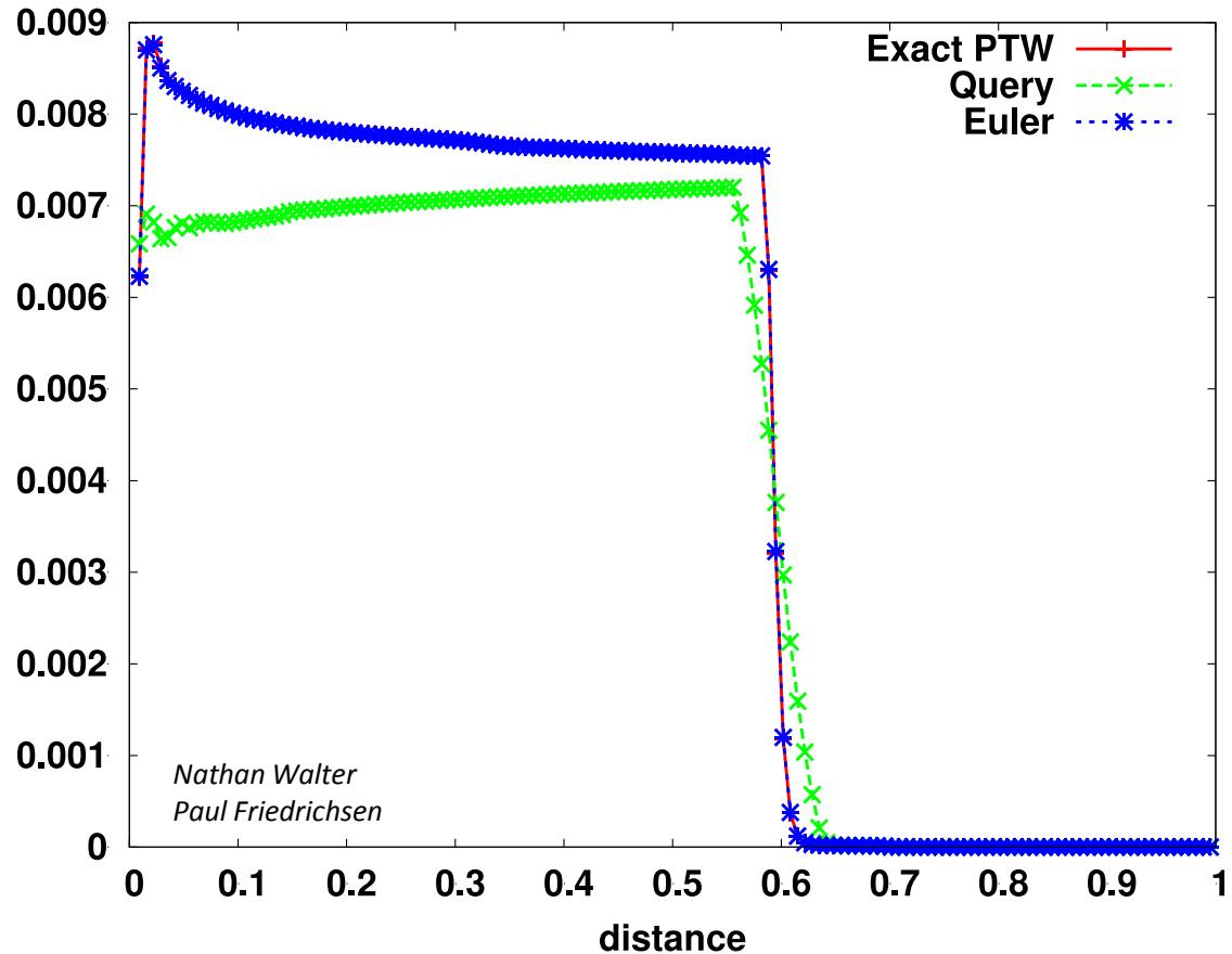
The figure shows that the exact PTW equation, when implemented correctly, is identical to Euler integration.
