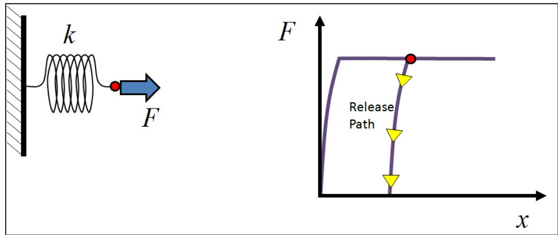
Determining how the plastic strain is related to stress is a central part of plasticity.
