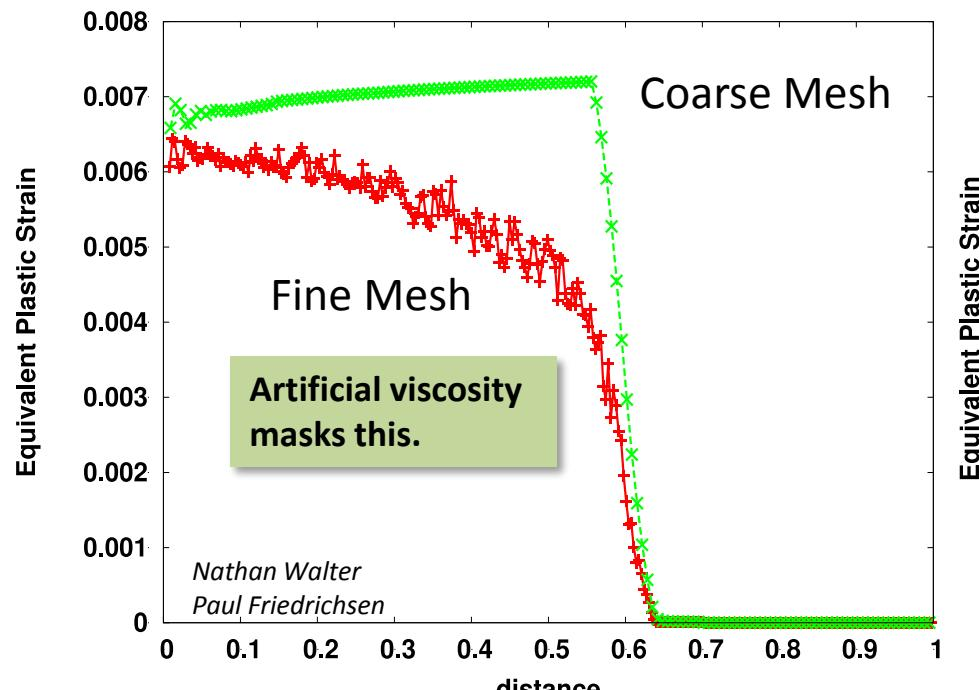
Discrete Radial Return with no iterations
