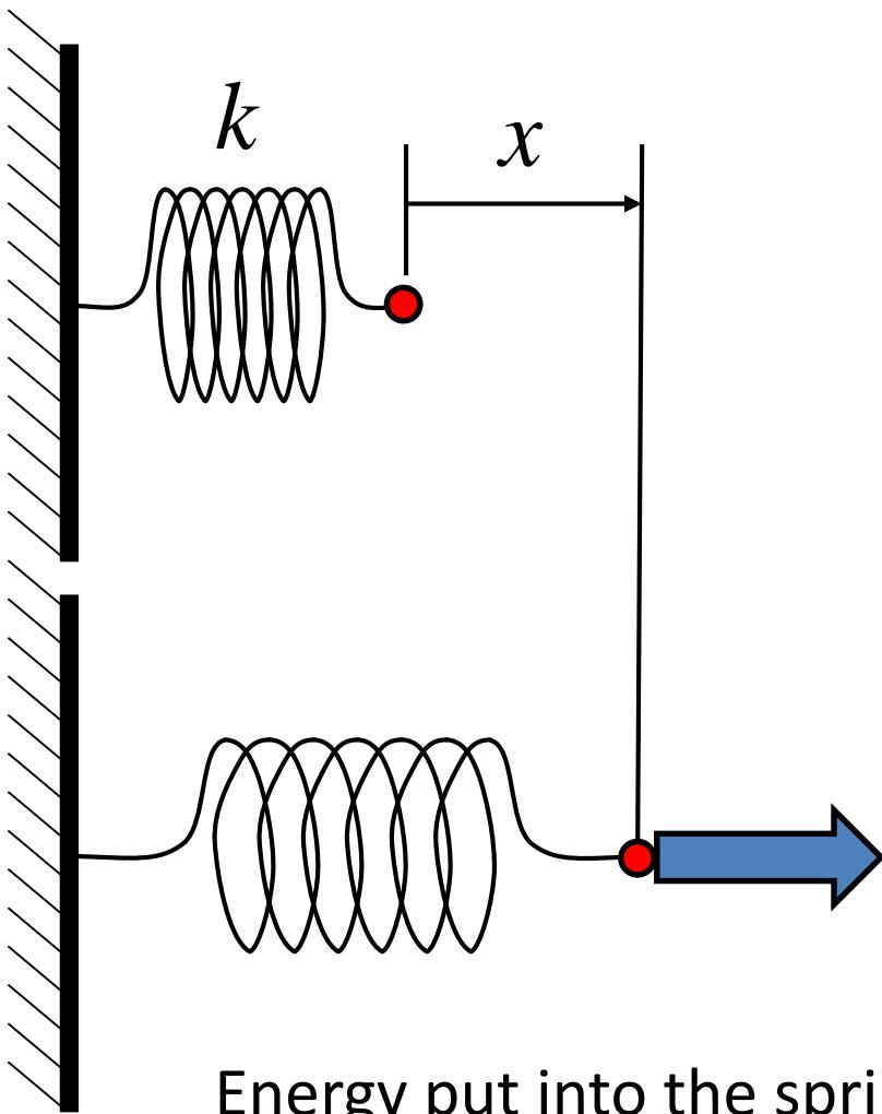
Energy put into the spring = Work = Force x Distance
