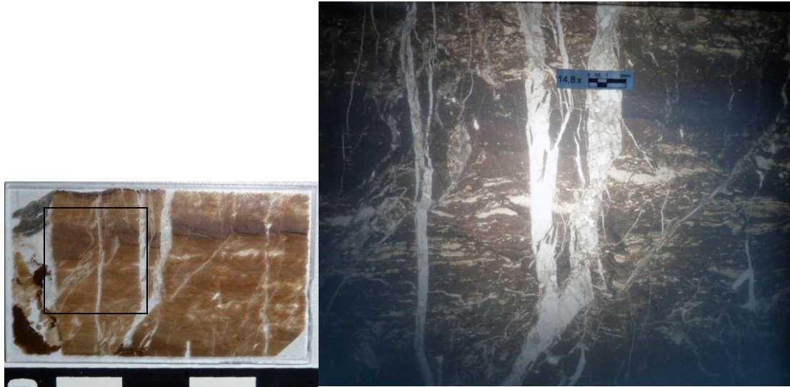
Figure 4-52 Picture of entire thin section and enlarged area showing the overall deformation
