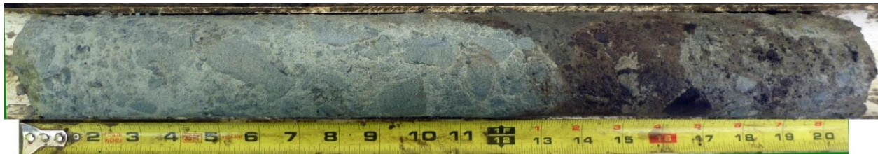
Figure 4-18. Sandstone protocataclasite at 629-632ft depth from WF4
