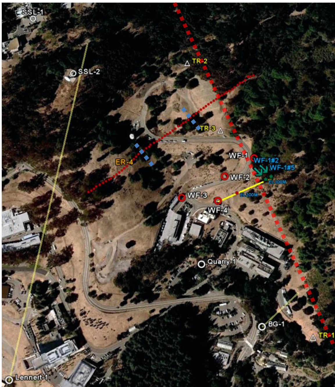
Figure 2-7: Location of ER-4 profile. The blue broken lines indicate potential fault trace identified in the ERT inversion. The red broken line is the previously suspected trace of the Wildcat Fault.
