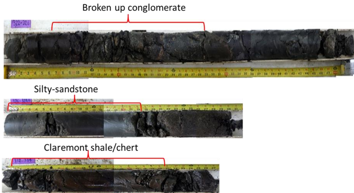
Figure 4-8 Zone of deformation characterized along the contact between Orinda Fm/San Pablo Gr. and Claremont Fm.
