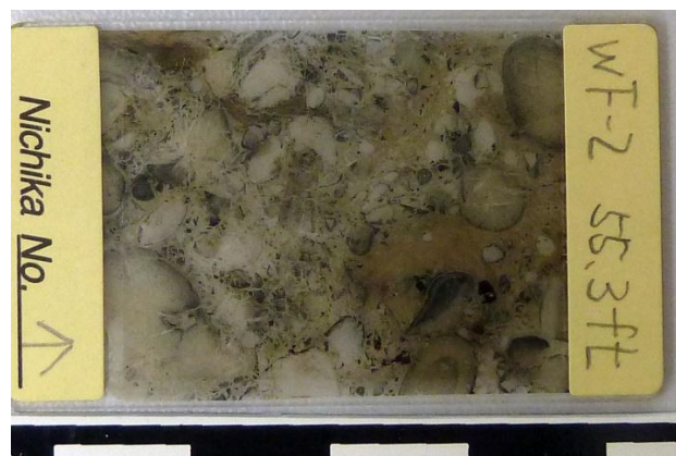
Figure 4-37. Thin section of WF2—16.8 m (55.3 ft), along the contact between Orinda Fm/San Pablo Gr. and Claremont Fm.
