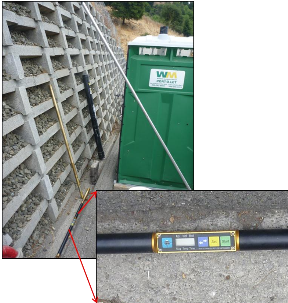
Figure 3-17. Borehole inclination survey equipment, with sensor probe enlarged. The 5 ft brass bar is the sensor housing that fastens to the 15 ft silver aluminum rod. An aluminum rod is attached to the wireline. The probe protrudes from the drill bit at enough distance away from the magnetically susceptible drill string.
