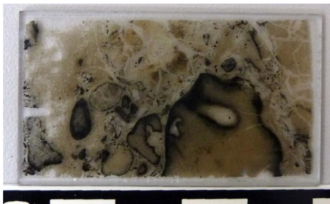
Figure 4-40. Thin section of WF3—98.75 m (321.9 ft) along the contact between the Orinda Fm/San Pablo Gr. and the Claremont Fm.
