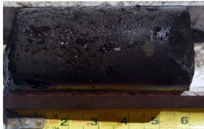
Figure 4-13. Example of carbonate concretions at WF4_23m (75ft )
