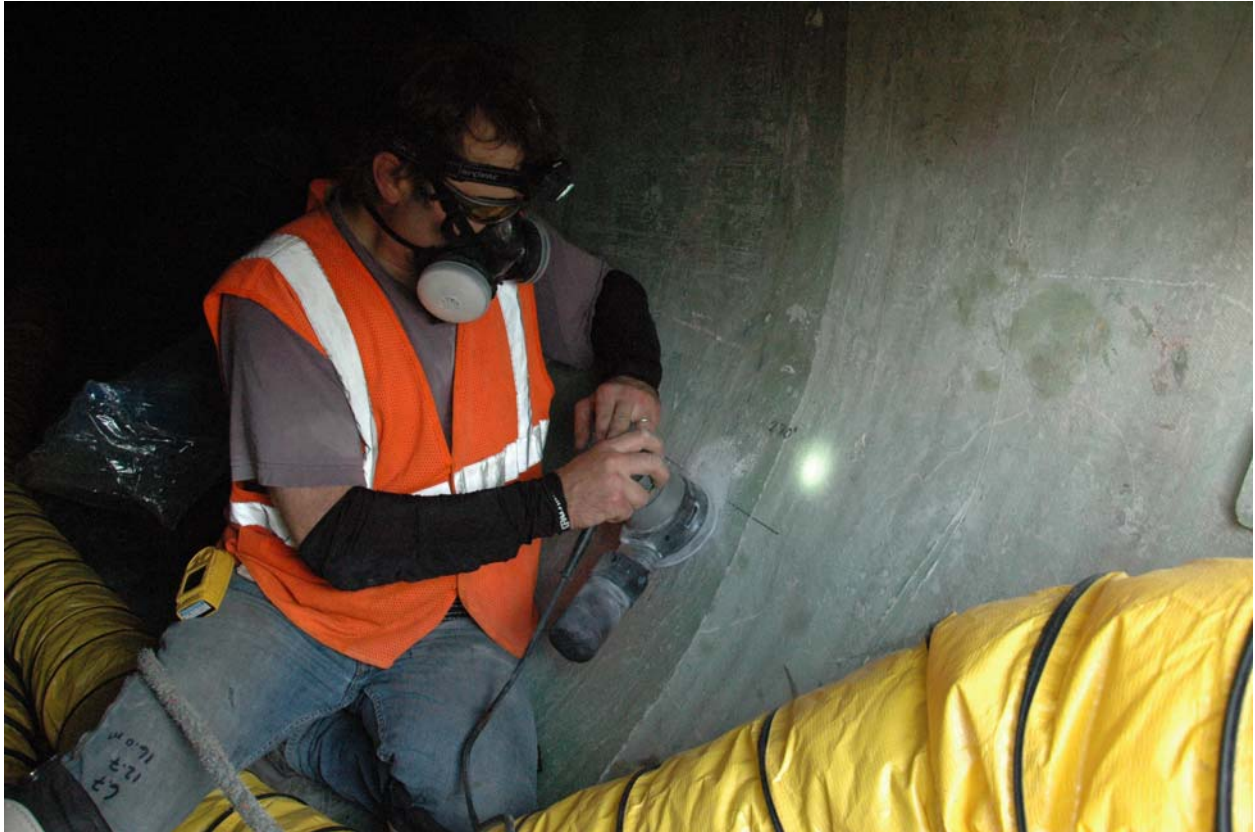
Figure 1.4: University of Minnesota research technician Dick Christopher prepares the inside surface of a wind turbine blade for the installation of fiber optic strain gauges and temperature probes.
