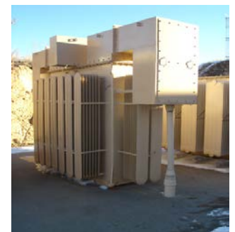
Refurbished Inductrol Voltage Regulators
