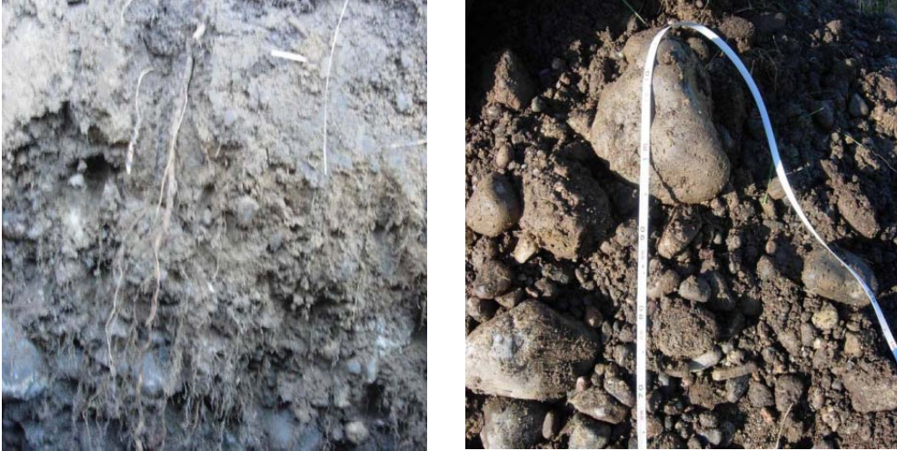
Figure 3. Typical sediments at the test site consisting of a thin unsaturated layer of mostly sandy silt with grass roots (left), underlain by a thicker saturated layer of coarse sand, gravel and cobbles (right).
