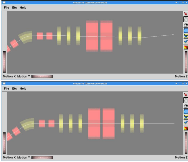
FIG. 36. The top figure shows a reference trajectory (28 MeV/c) with the field of D3 too low by a factor of 0.94 ( Bd3=0.052088 T). The bottom figure shows the reference trajectory with correct field of Bd3=0.055413 T.
