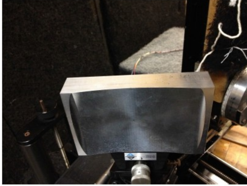
Fig. 35. Input mirror mounted on a series of positioners.
