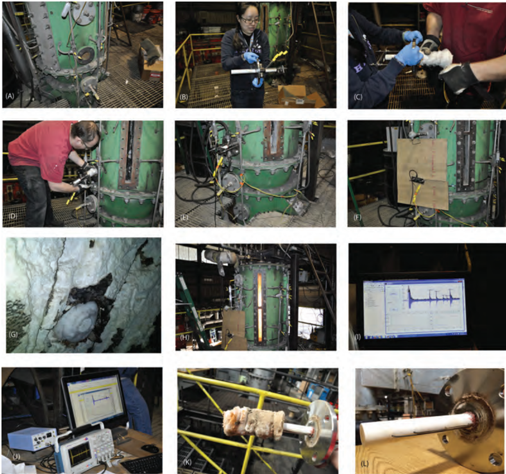
Figure 6.5: (A) Waveguide was mounted in P3 port. (B) Engineered alumina waveguide is shown mounted in the flange fixture. (C) Thermal insulation was wrapped around the waveguide. (D) The fixture is being inserted into P3 port. (E) The mounted waveguide is shown with the attached ultrasound transducer connected to the BNC cable leading to the US data acquisition system. Thermocouples are shown connected to DAQ. (F) Radiation shield is now installed. (G) Distal end of the transducer is shown to be mounted flush with the refractory surface. The picture was taken prior to the experiments with a camera inserted inside the ignition zone. (H) The system during the experiments. (I) Computer screen shows the ultrasound waveforms acquired in real time and the corresponding temperatures obtained with ultrasound measurements. (J) Components of the ultrasound data acquisition system. (K) The waveguide removed from the port at the completion of the experiments. (L) The waveguide after removing thermal insulation. Note thermocouple wires inserted into holes drilled to provide US echoes.
