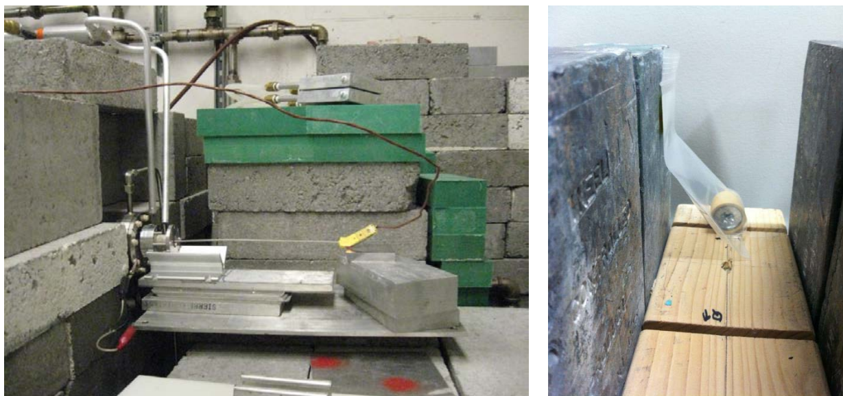
Figure 13. Zn irradiation setup. Thermocouple is inserted for temperature measurements. Cold air is blowing on both converter and target.
