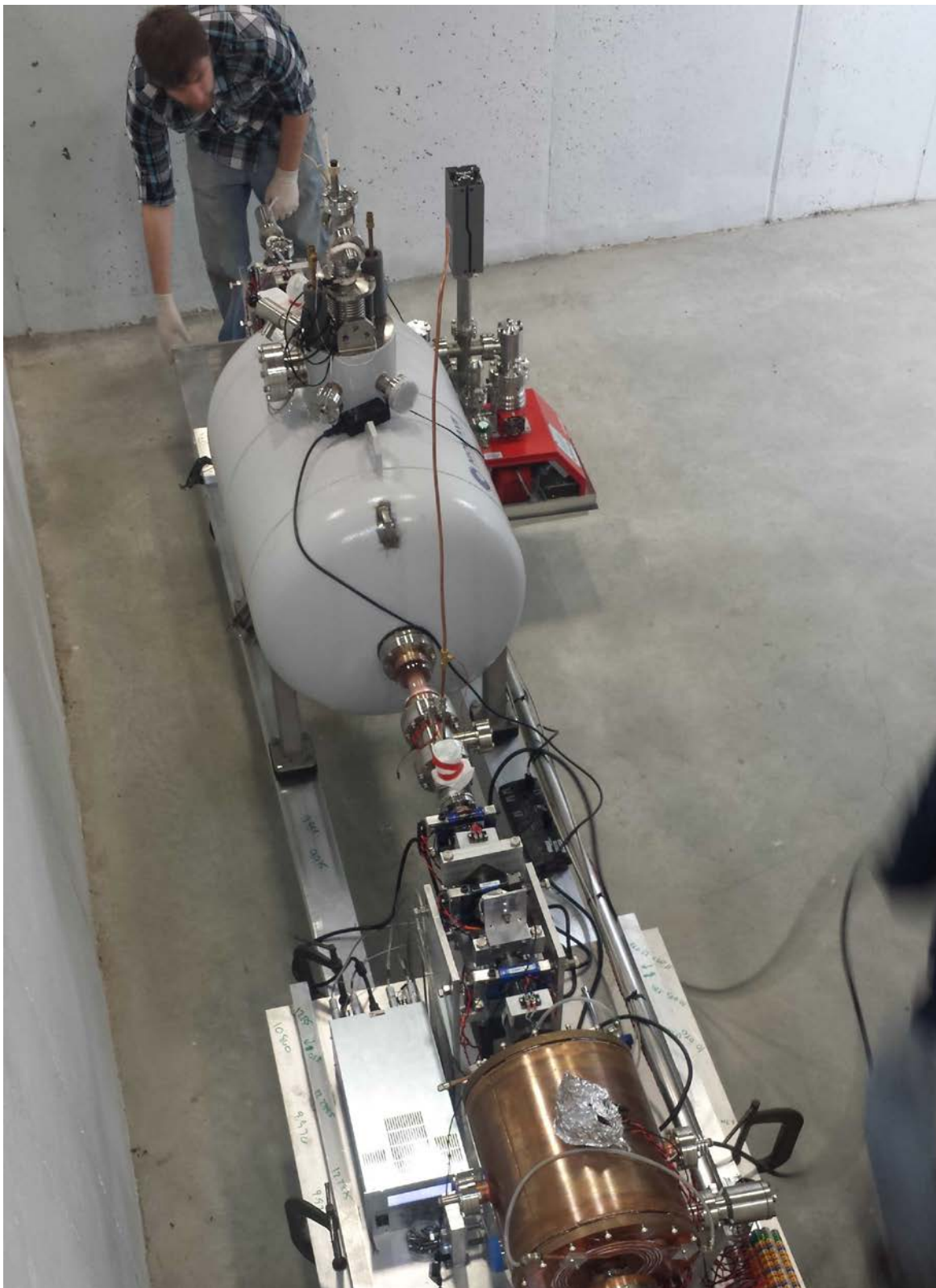
Figure 2. A single-cell cryomodule with normal-conducting electron gun and beamline being installed into the testing tunnels at Niowave for first beam testing.
