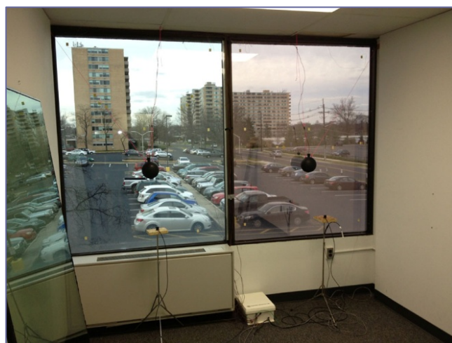
Figure 14: South-facing test office. Low-E retrofit system on left, original single pane window with silver window film on right.
