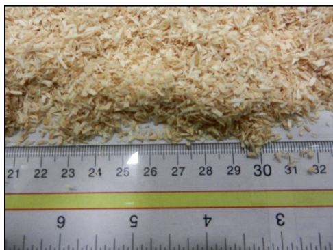
Figure 4. Sawmill Pine dimension is in the 1/16" to 1/8" range
