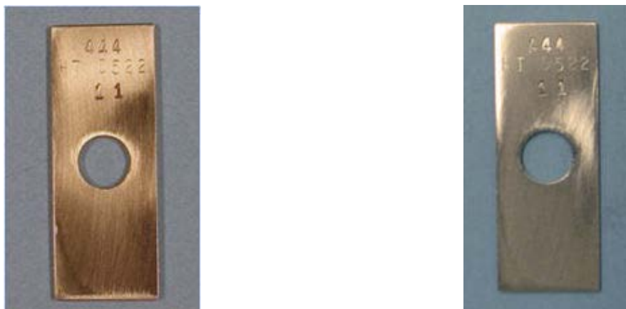
Figure 34. Before (left) and after (right) image of a 444 sample coupon after 1,000 hours of exposure to pyrolysis oil heated to 50°C.
