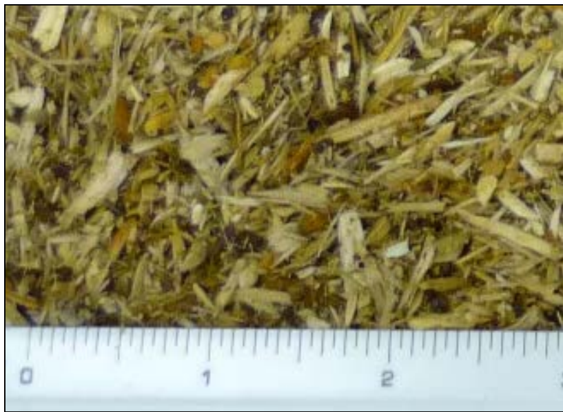
Figure 7. Particle size distribution from pulp and paper mills is in the range of 1/8" to 1/2"
