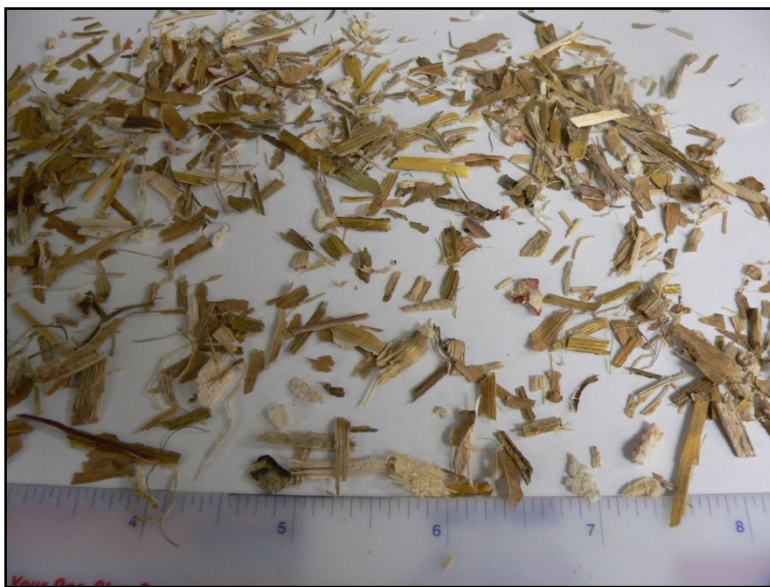
Figure 18. Particle size distribution for corn stover is in the range of 1/8" to 1/2" with some lengths approaching 1"
