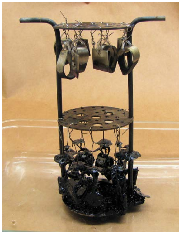
Figure 41. The appearance of the sample rack and samples after the 1,000-hour autoclave test conducted at 155°C.
