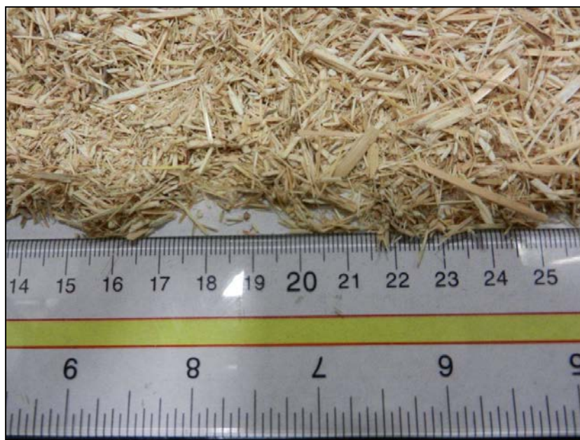
Figure 9. Particle size distribution of Miscanthus is in the range of 1/8" to 3/4"
