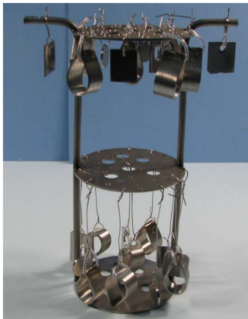
Figure 40. Test stand used to suspend samples during the autoclave exposure. The samples at the top of the sample rack were exposed to the vapor space while samples at the bottom were submerged.
