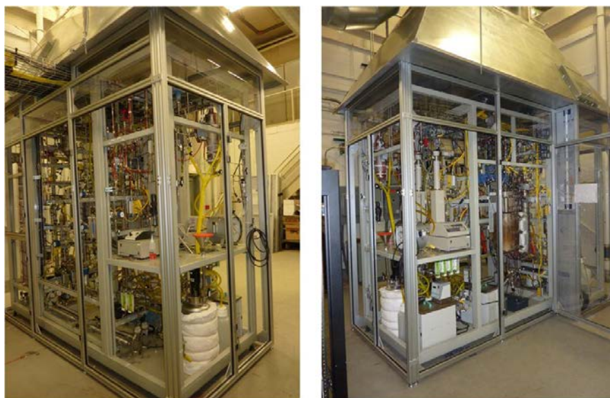
Figure 25. Front and Rear views of the Battelle Hydrotreatment System, shown fully installed with ventilation system and enclosure
