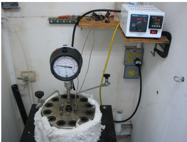
Figure 39. The autoclave test setup with temperature controller.
