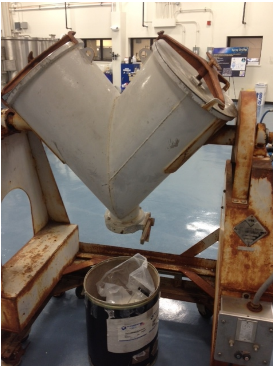
Figure 10. The V-blender used to successfully scale up PCM powder coating
