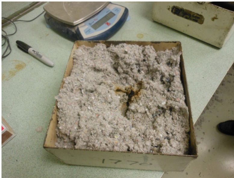
Figure 9: ASTM C793 Sec 14 Smoldering Combustion Test on (30 wt% graphite-PCM + cellulose insulation) sample.
