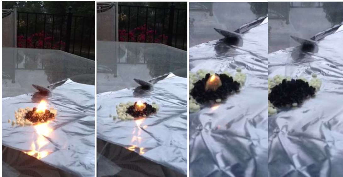
Figure 13. Sequence of images showing that the PVDC-coated PCM pellets self-extinguish after being set on fire. The time from start of fire until it extinguished was about six minutes.
