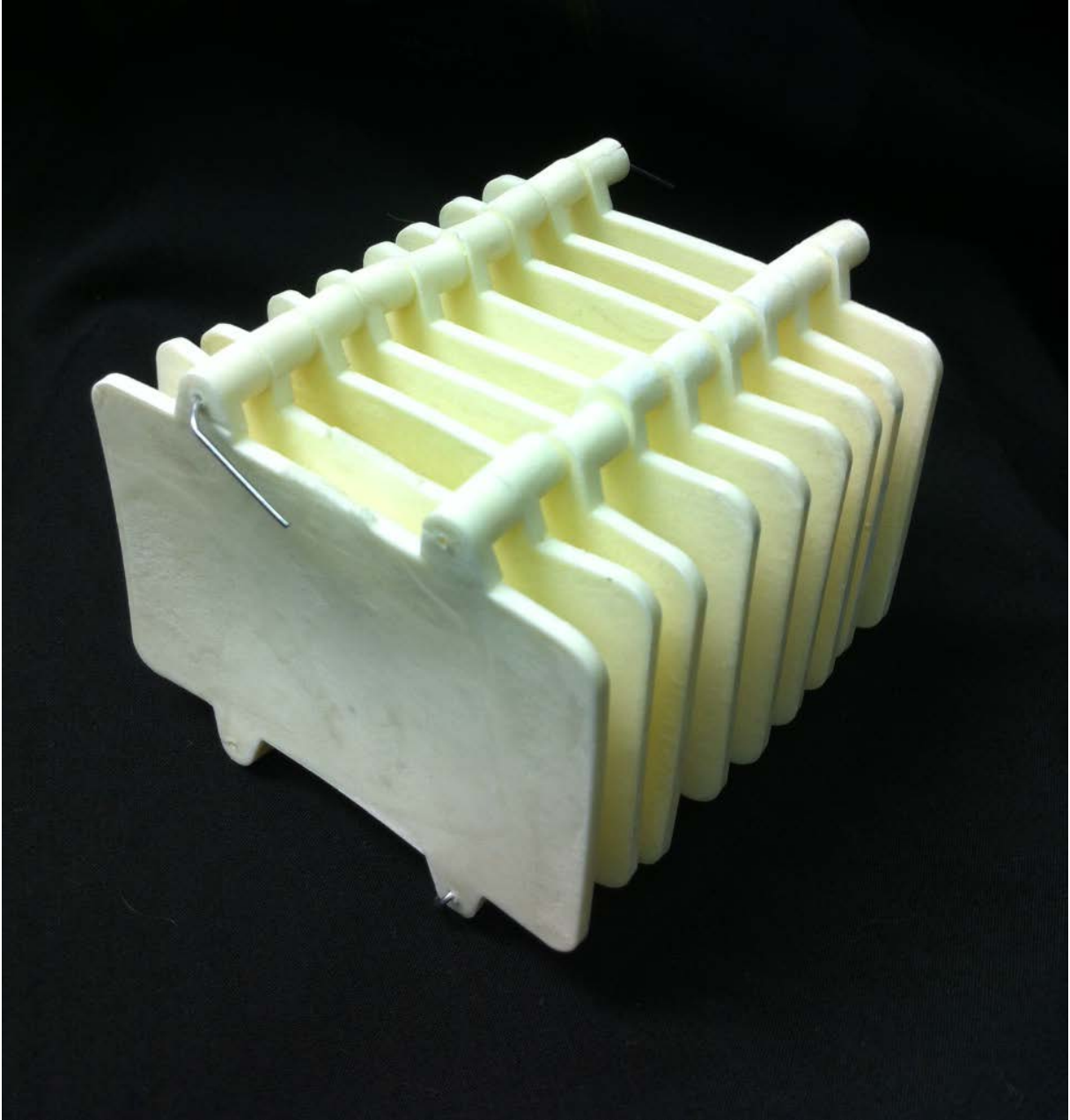
Figure 14. Prototype of parallel-plate thermal storage device suitable for air handling systems. The plates are made by injection-molding the low-cost PCM composite.
