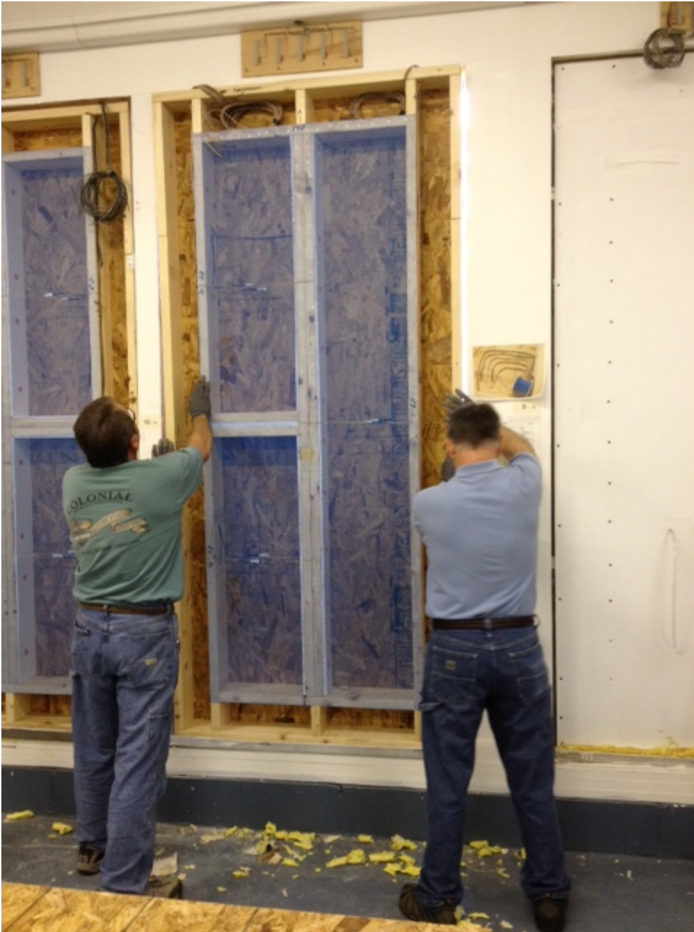
Figure 11. Installation of wall for field test. The wall cavities were filled with cellulose insulation, and two configurations of PCM-modified cellulose insulation.
