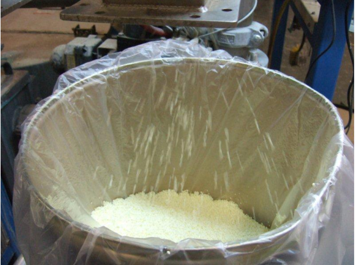
Figure 3. PCM pellets (~2 mm) coming off of the compounding/pelletizing line
