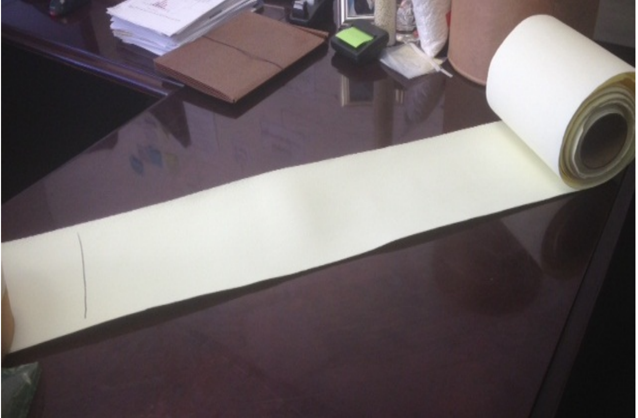
Figure 15. Prototype of PCM sheet for lamination to wallboards and other building envelopes. The sheet was prepared by extrusion of the low-cost PCM composite.
