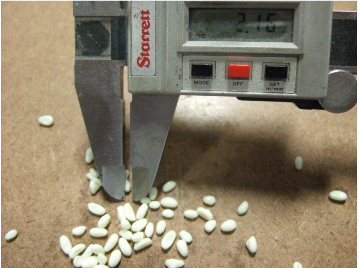
Figure 4. PCM pellets measure about 2 mm
