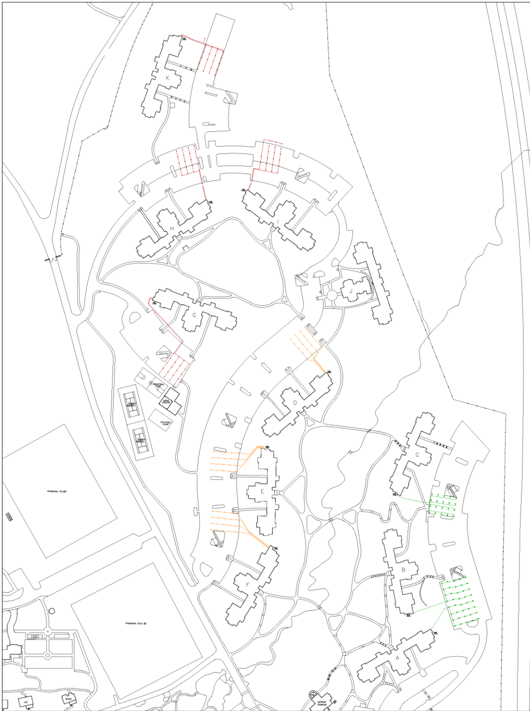
FIGURE 2 - This diagram displays the layout of the geothermal well fields for all apartment buildings that were renovated. Each dot represents a well that is connected to the building's geothermal ground loop.
