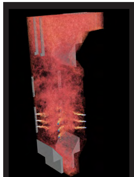
Figure 2. Volume rendered image of the concentration of the smaller (20 micron) particles in the Alstom 50 MW pilot scale oxy-coal boiler. The simulation and visualization details are the same as those specified in the Figure 1 caption.
