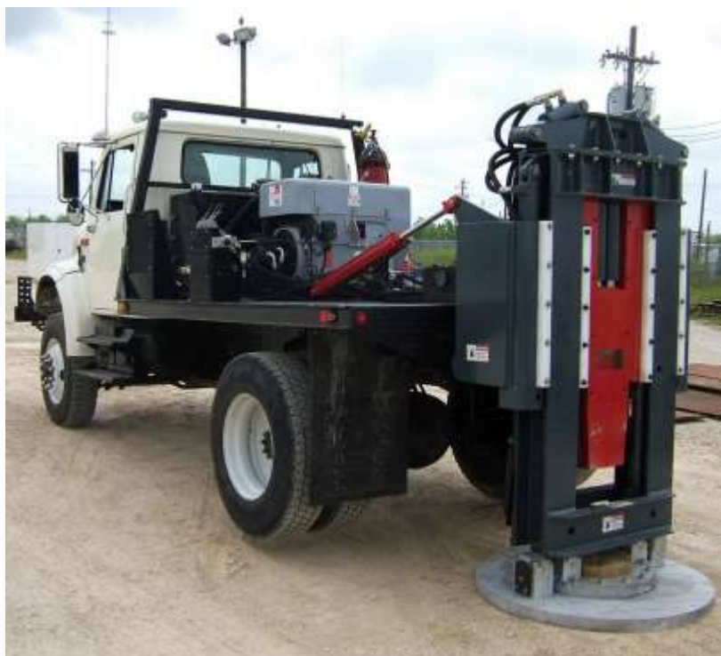
Figure 2: An AXIS accelerated weight-drop seismic source with 500,000 ft/lbs of energy per shot was used for the seismic surveys.
