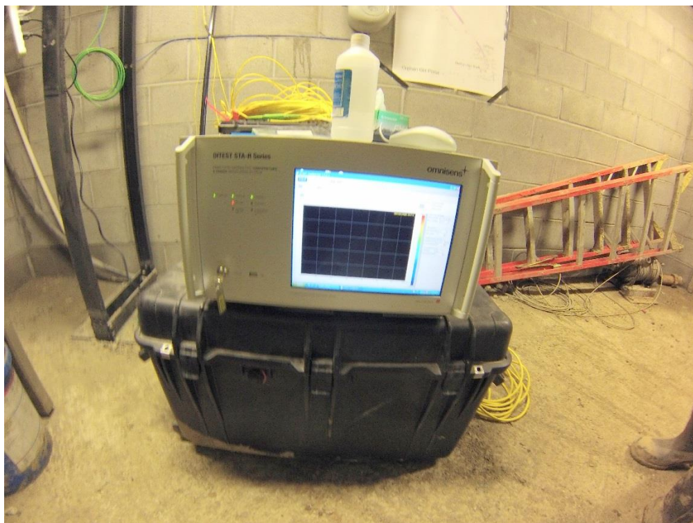
Figure 4. Pictured above is an Omnisens DITEST STA-R™ high-performance Brillouin-based fiber optic distributed temperature and strain analyzer collecting temperature data in the Orphan Boy mine shaft.
