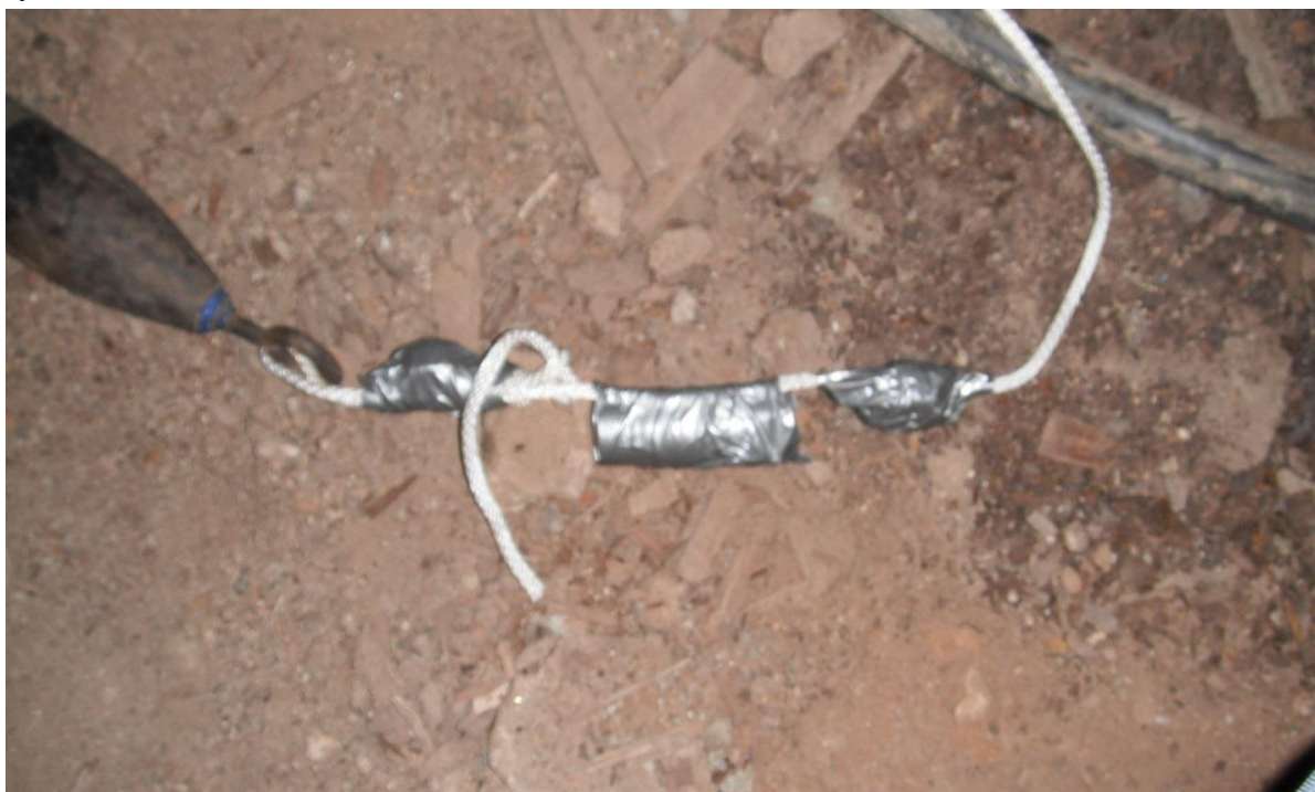
Figure 5. Pictured here (from left to right) is: one 20 kg slug, one Hobo Tidbit temperature logger, one Star-Oddi Seastar DST CTD miniature salinity/temperature/depth logger, another Hobo Tidbit, and 2000 feet of 3/8" nylon rope.
