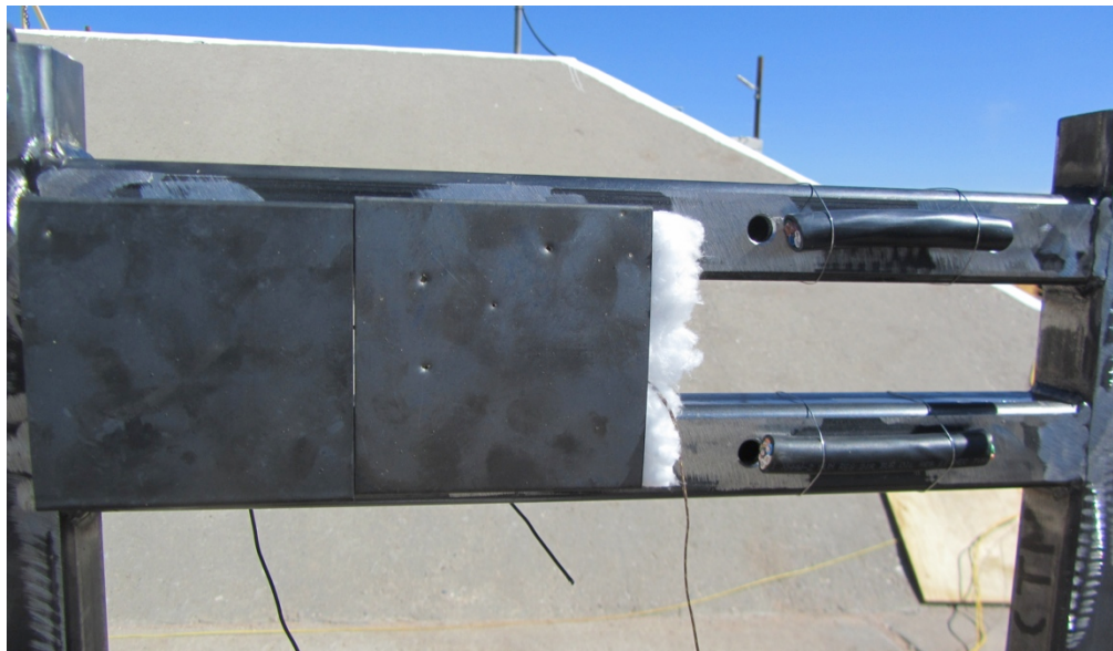
Figure 27. Damage to a plate thermometer during Test Arc-01
