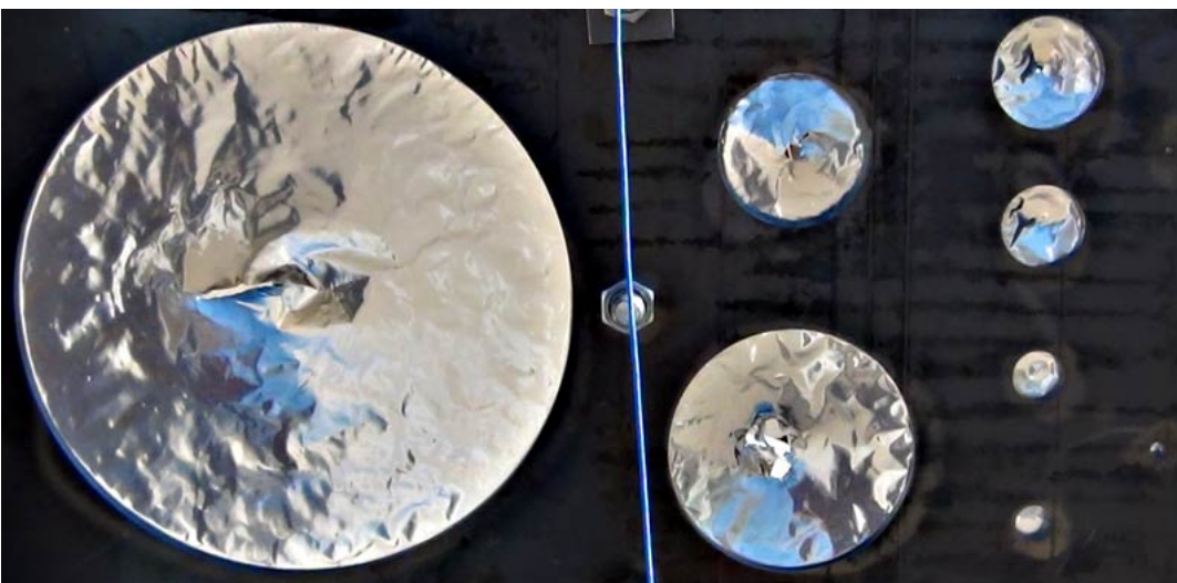
Figure 31. Arc-03 Bikini Gauge Results for 3 (top), 6 (middle), and 9 ft (bottom)
