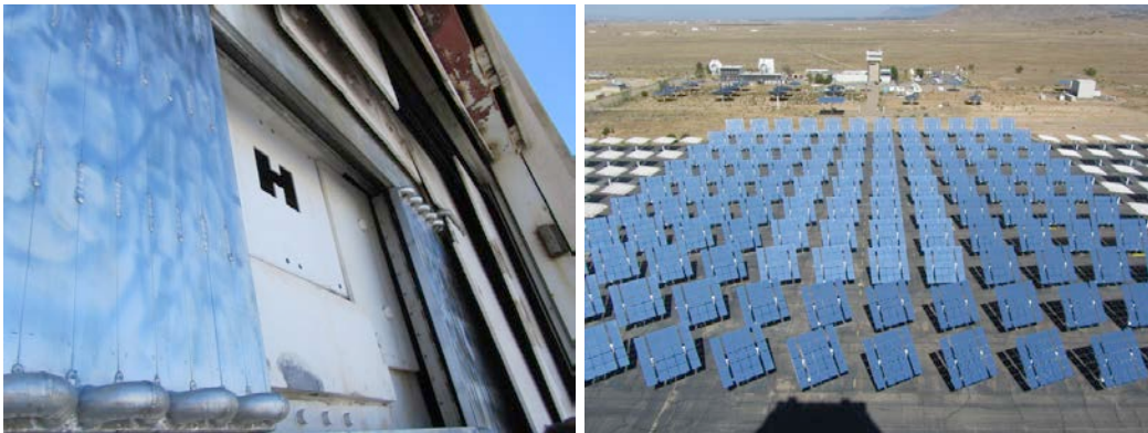
(c) Shutter in the open position (left) and array of heliostats used for these tests (right)
