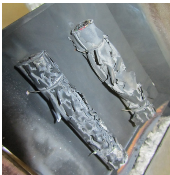
Figure 24. Close-up of cable segments after Test 7 (thermoset left & thermoplastic right)
