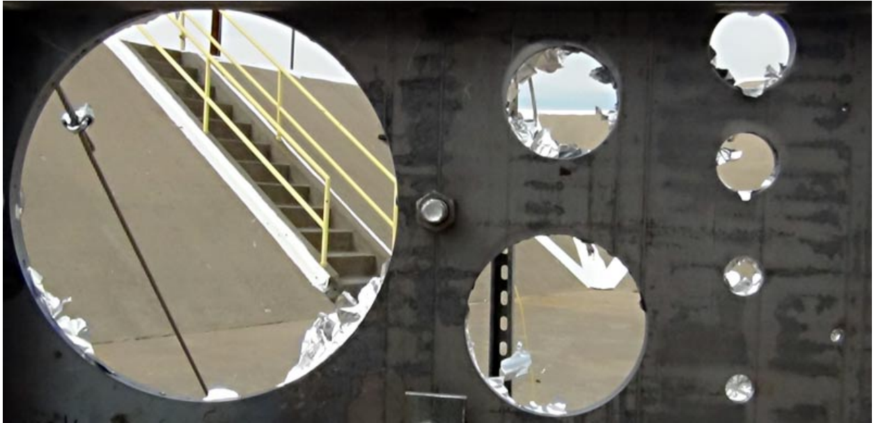
Figure 28. Arc-00 Bikini Gauge Results for 3 ft
