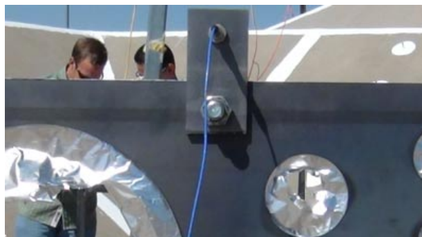
Figure 26. Set-up for Tests Arc-01 - 03 (top); Test Arc-04 (middle); reflected pressure gauge mounted on the Bikini gauge (bottom)
