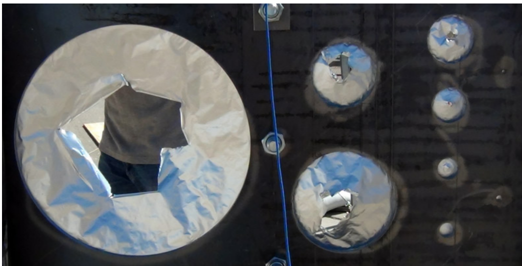
Figure 29. Arc-01 Bikini Gauge Results for 3 (top), 6 (middle), and 9 ft (bottom)
