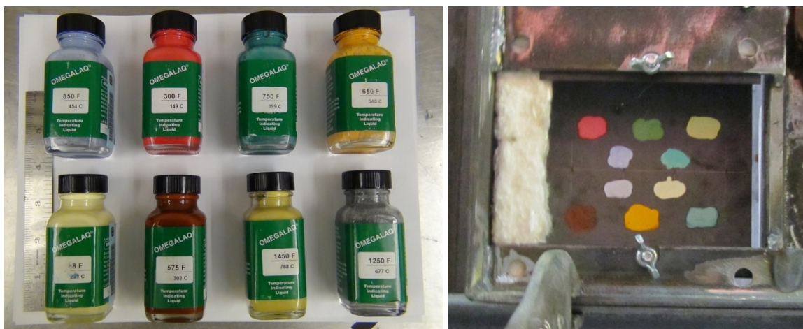
Figure 2. OMEGALAQ ® liquid temperature indicators in bottles (left) and as applied on thin plate (right)
