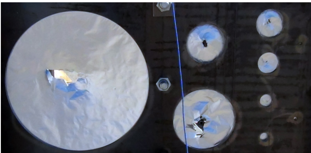
Figure 30. Arc-02 Bikini Gauge Results for 3 (top), 6 (middle), and 9 ft (bottom)
