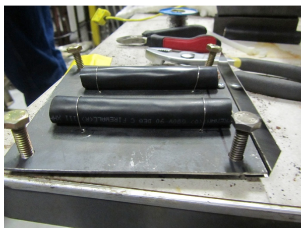
Figure 3. 9 cm (3.5 in) long cable segments (one thermoset and one thermoplastic)
