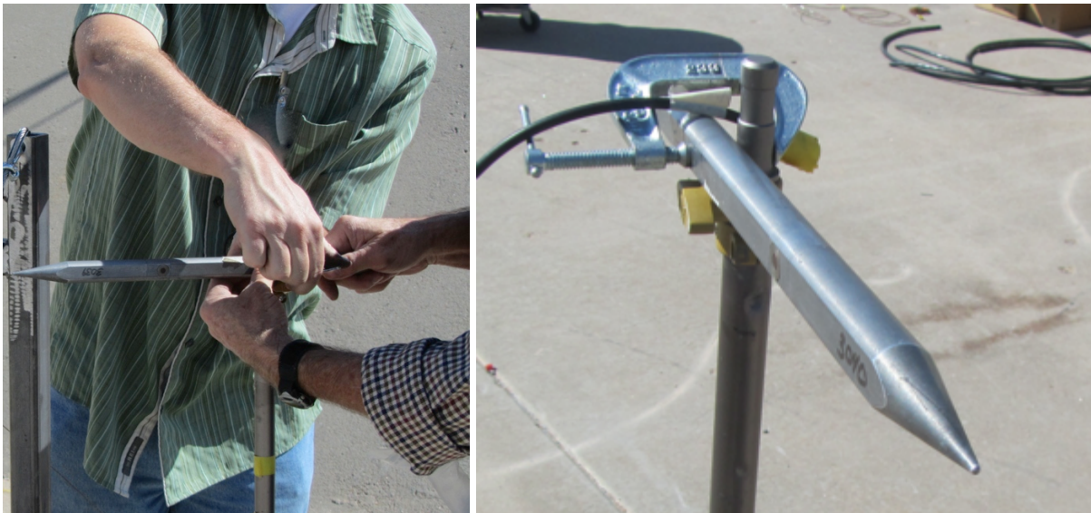
Figure 9. Pressure transducer: Pencil gauge being installed on a tripod before testing (left) and as installed on tripod (right)
