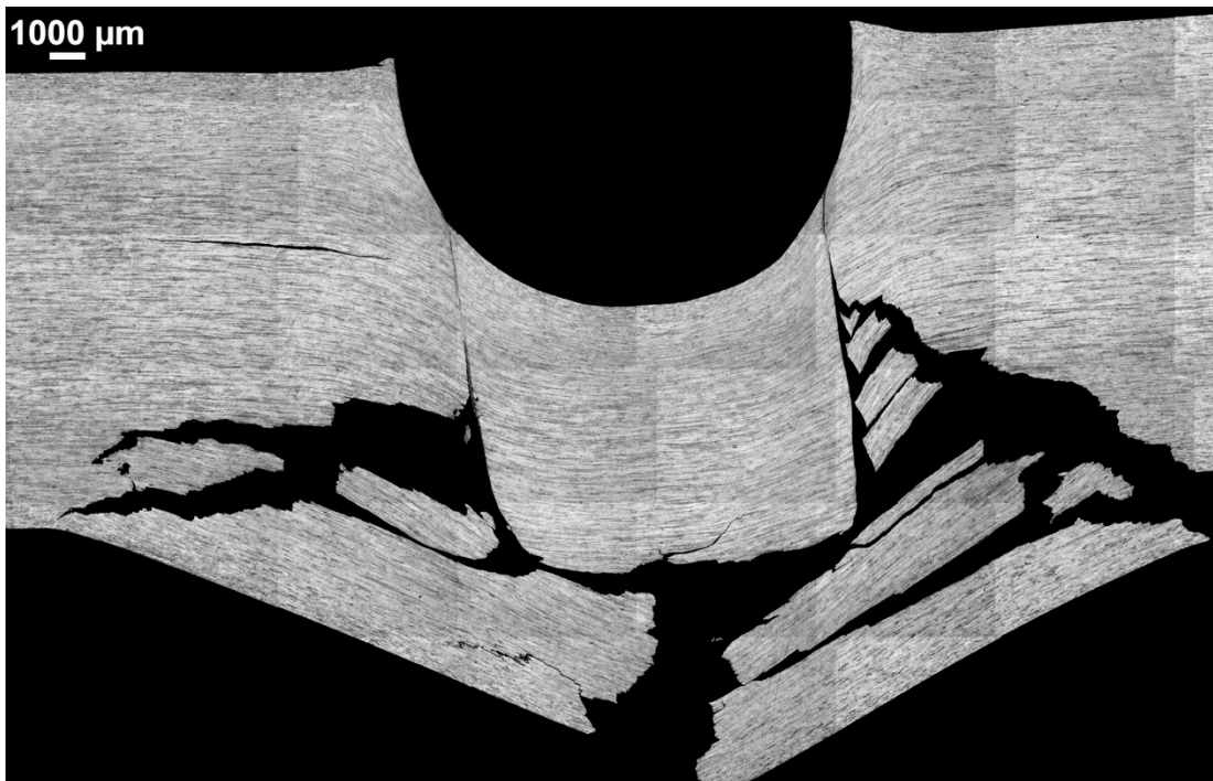
Figure 6: Section of specimen 13 through the center of the impact dimple.
