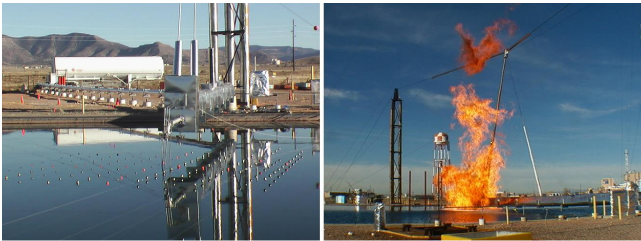
Figure 9. LNG Free Spillage Pool Fire Testing at WIF
