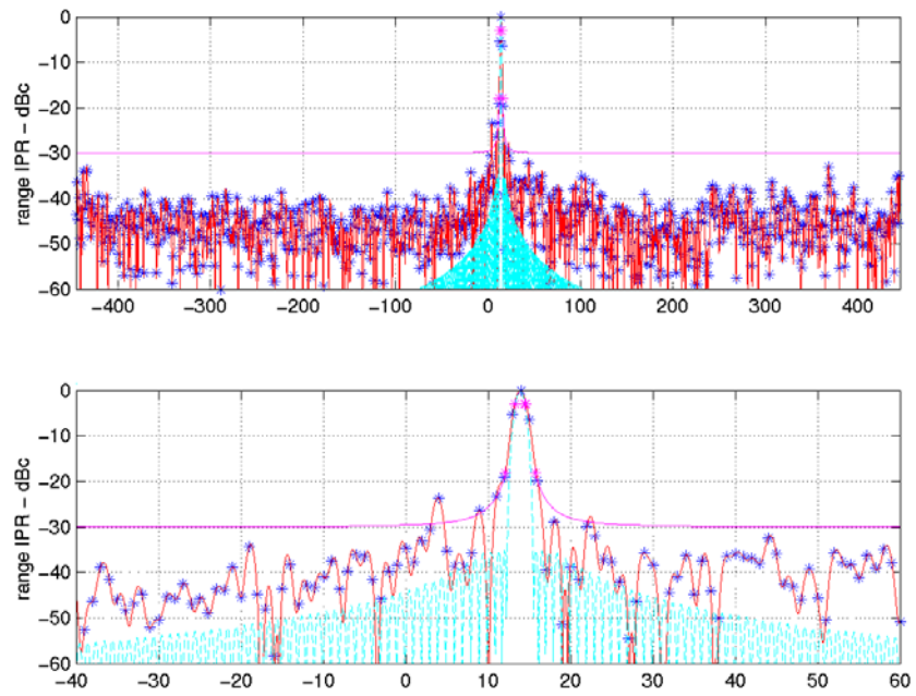
Figure 12. Range slice of ARF processed image.
