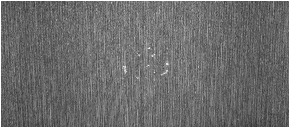
Figure 1. SAR image corrupted by interference.
