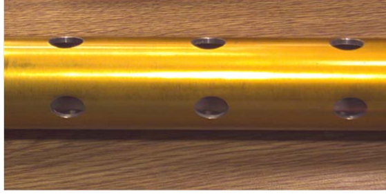
Figure 4. Cylindrical shield with periodic set of four circumferential circular apertures.
