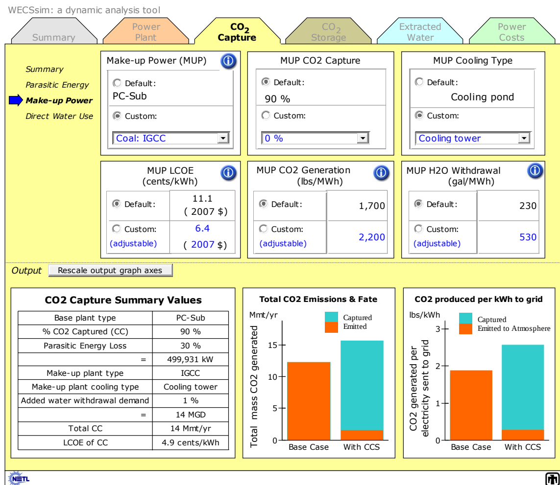
Figure 29. Scenario specifying IGCC with cooling towers for all make-up power.
