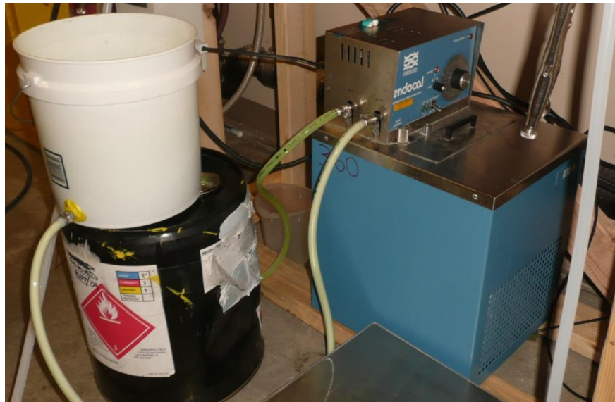
Figure 23: Endocal heater/chiller with heat transfer bucket and tubing attached.
