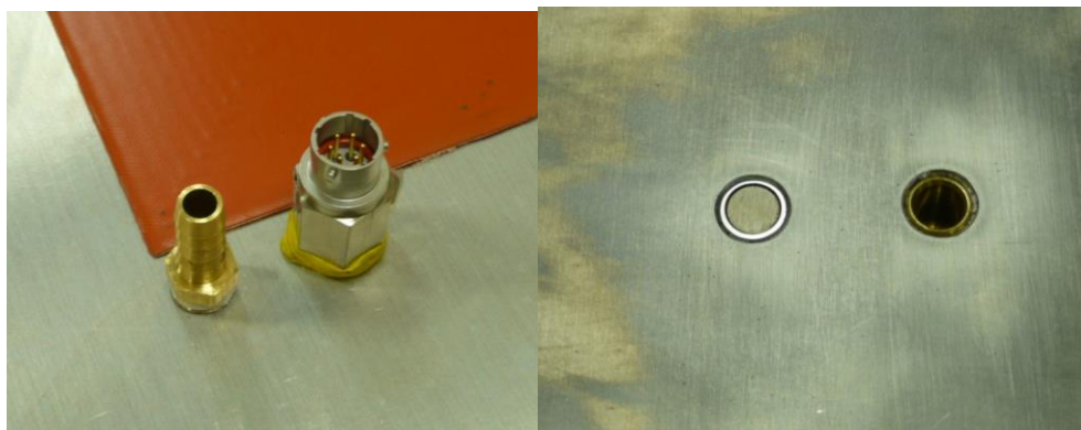
Figure 27: Mounting the transducers to the aluminum mold.
