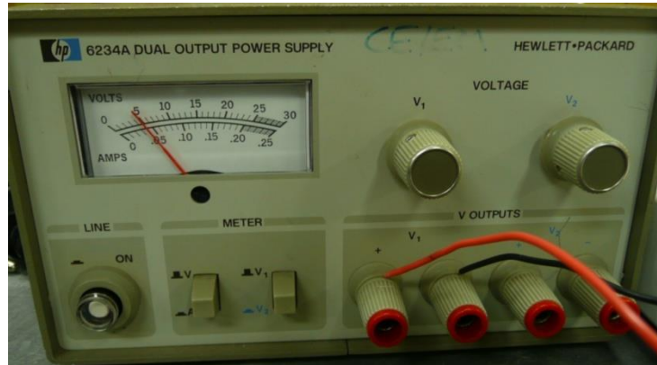
Figure 28: 6234A dual output Hewlett Packard power supply used to power the pressure transducers.
