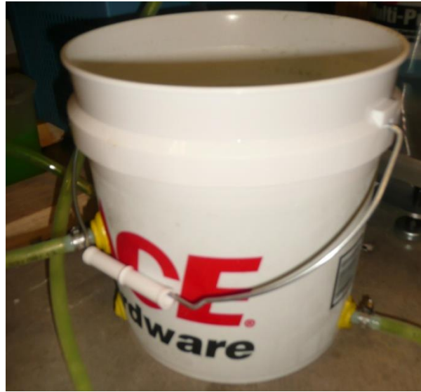
Figure 22: Heat exchanger bucket for heating or cooling the resin.
