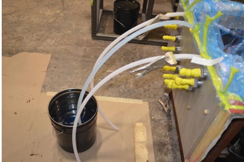
Figure 11: Resin is mixed in large pails, and then transferred to 5-gallon buckets during the injection process. Modified, vise-grip clamps are used to control the flow of resin and to seal the vacuum and injection tubes when not in use.
