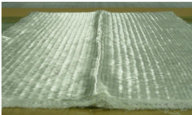
Figure 52: Laminate 2333 manufactured with a small amplitude and steep angle OP wave.
