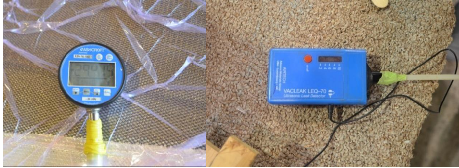
Figure 9: Leak detection techniques include monitoring the quality of the vacuum over a period of time using a pressure gage (left); as well as an ultrasonic leak detection device (right).
