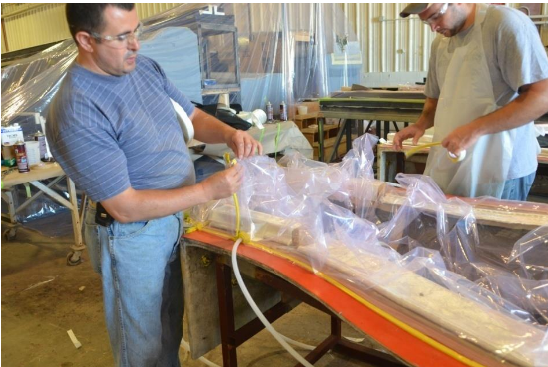
Figure 8: Technicians at TPI applying vacuum bag to the mold of one half of a BRC blade.
