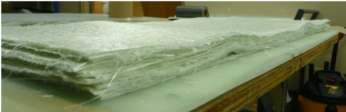
Figure 51: Out-of-plane waves inserted into 20 layers of uni-directional fabric using Super 77.
