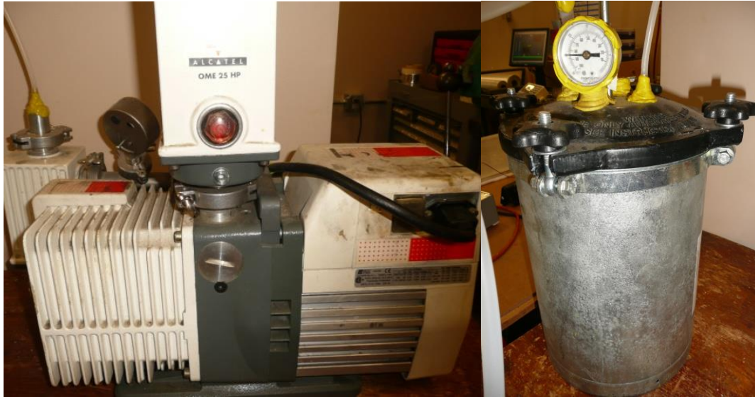
Figure 24: Alcatel Industrial vacuum pump and resin trap.
