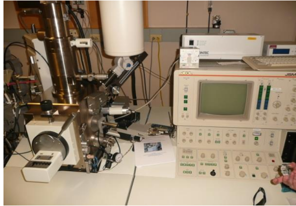
Figure 41: Scanning Electron Microscope (SEM) used for analyzing porosity samples.
