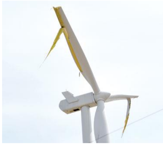
Figure 13: Wind turbine blades manufactured by Vestas which suffered failure due to manufacturing defects, [25].
