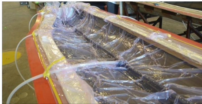
Figure 10: Completed laminate under vacuum seal and ready for resin injection.
