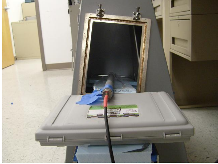
Figure 3.2. GTEM Cell Field Measurement View 2.
