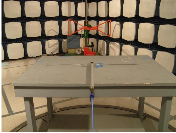
Figure 3.9. Chamber Field Measurement Setup.
