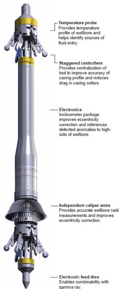
Figure 47: Weatherford's multi-sensor caliper [Weatherford, 2010]
