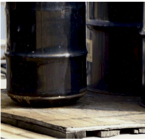
Figure 1. Severely over-pressurized closed-top drum. Note how the bottom is bulging. Source: Y-12 National Security Complex
