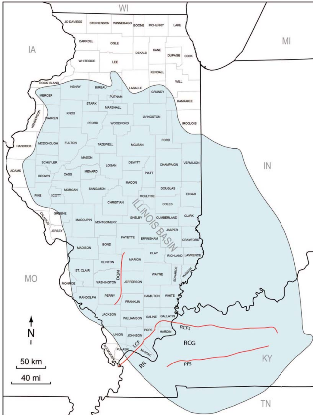
Figure 1: location of the Illinois Basin in light blue (Buschbach and Kolata, 1991); LCF: Lusk Creek Fault; PFS: Pineville Fault System; RR: Reelfoot Rift; RCG: Rough Creek Graben; RCFS: Rough Creek Fault System (Fault trace after Kolata and Nelson, 1991).
