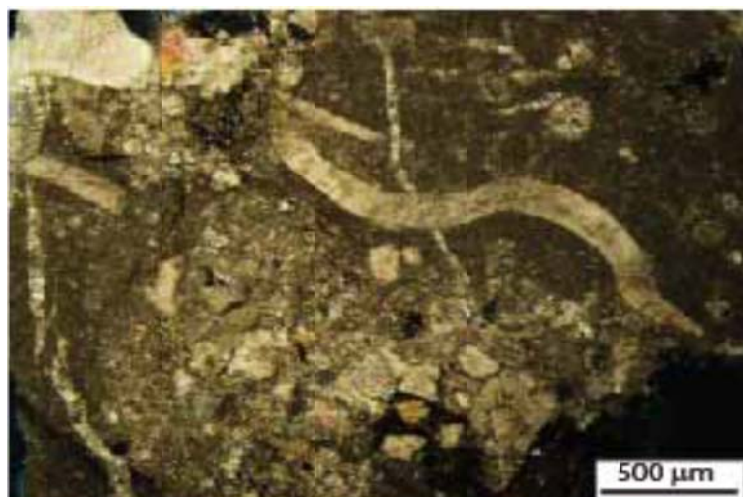
Fossiliferous lime mudstone to wackestone with trilobites, crinoids, pellets under plane light; Thin section photomicrograph from Conoco Inc. Dyhrkopp No. 4-1, Gallatin Co. IL; (depth 13650-80 ft).
