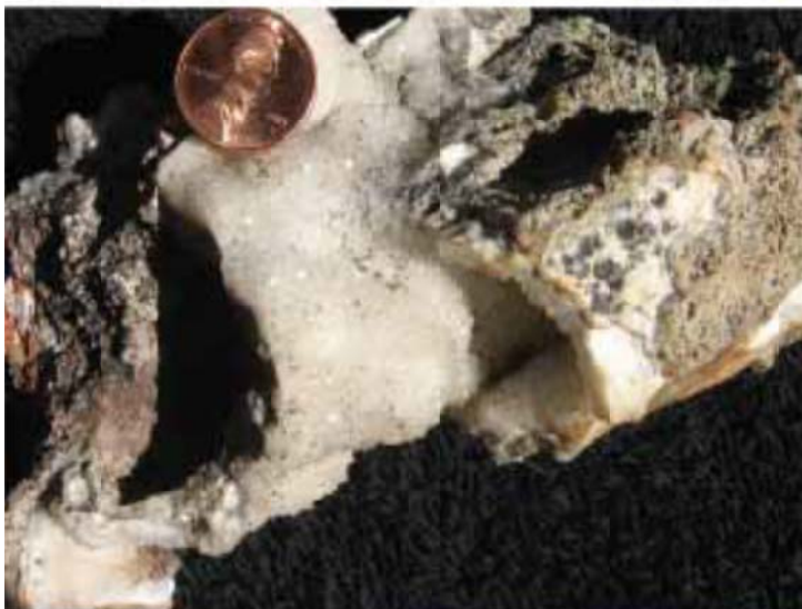
Hand sample of drusy quartz in the Potosi dolomite. Junction Highways 21 and 47, south of Potosi, MO.
