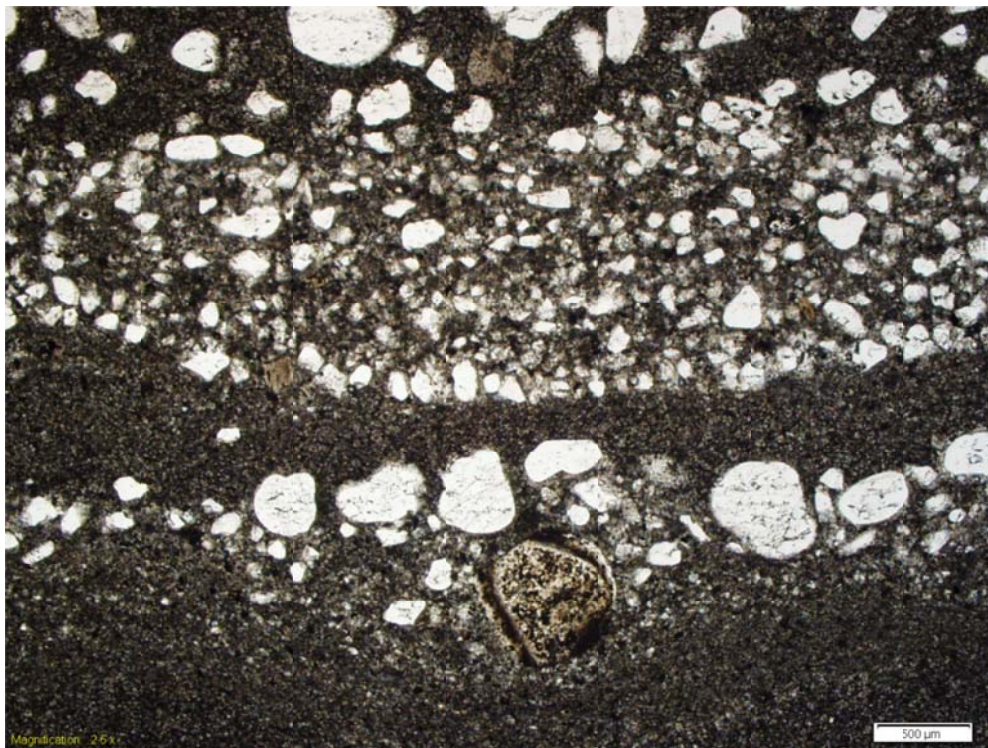
Figure 2. Photomicrograph of Morgan Co., IL, Gunter Sandstone sample C-13687-2485.2', a micrite (fine gray matrix) with interbedded quartz (larger colorless grains) laminations.
