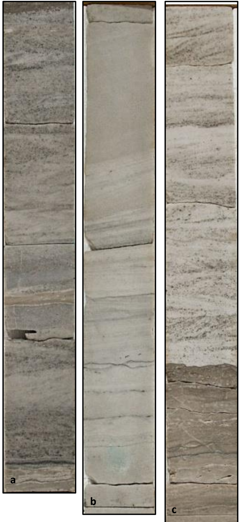
Figure 2-11. Quartz sandstone lithofacies, all from KGS 1 Blan well, New Richmond interval, core width = 4 in (10 cm)
