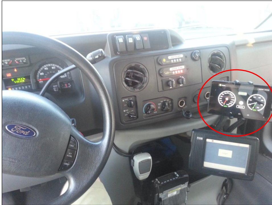
Figure 5-3. Driving feedback system installed in RTA shuttle
