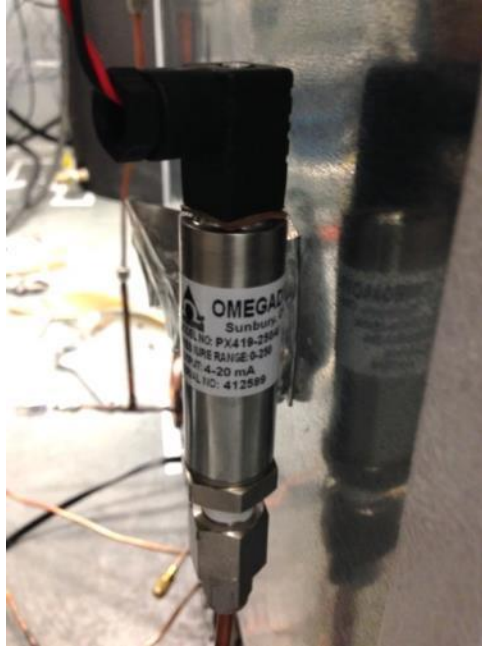
Fig. 2.13: Pressure transducers used in the test
