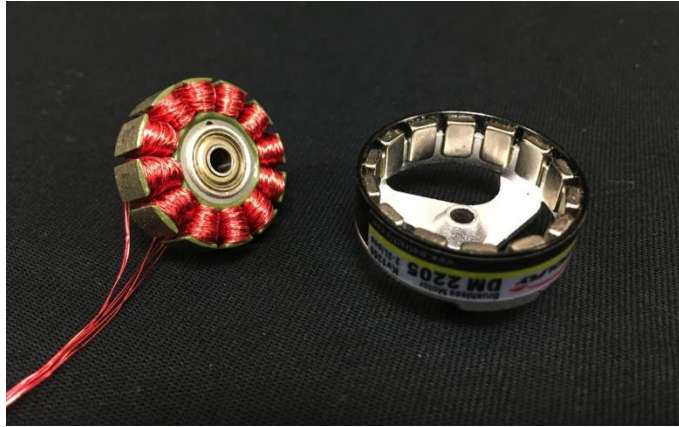
Fig. 3.14: Motrolfly motor assembly
