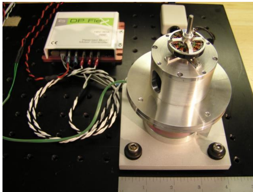
Fig. 3.17: Hysteresis Brake setup
