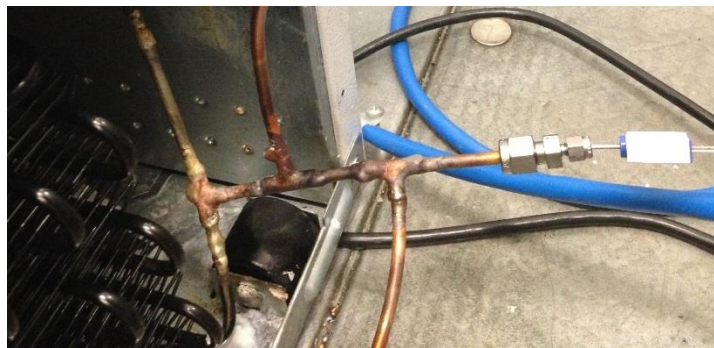
Fig. 2.8: Instream thermocouple for refrigerant side temperature measurement
