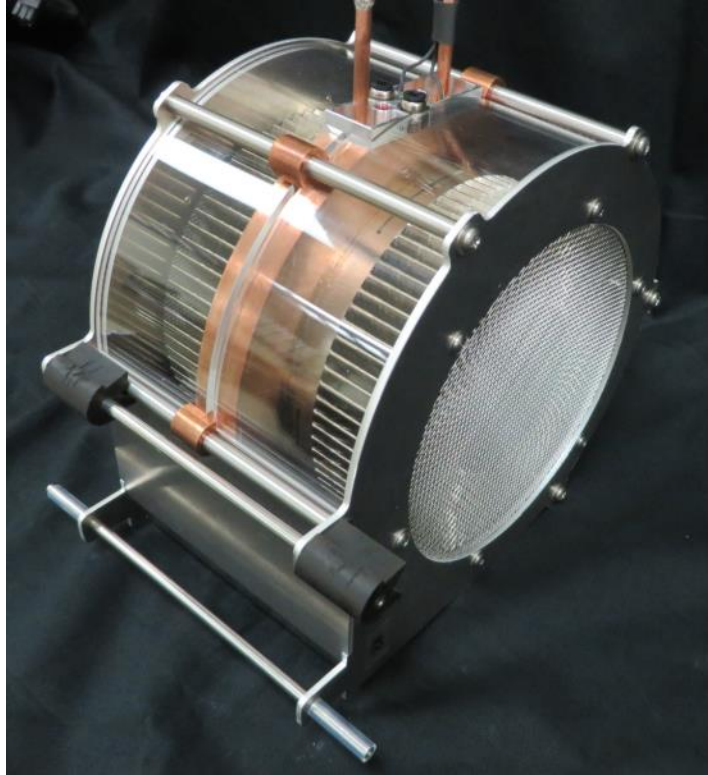
Fig. 3.28: Fully assembled Sandia Cooler condenser
