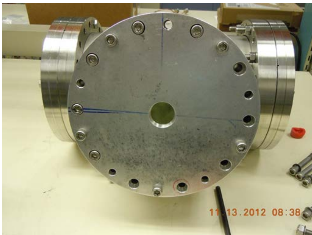
Figure 20. The vacuum test chamber showing aperture allowing radiation exposure of samples
