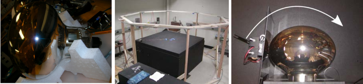
Figure 6: Hamamatsu R11781 12" PMT, designed for LBNE (left), Penn PMT testing darkbox and magnetic compensation coils (center) and LaTorre's automated scanning arm with opaque pinhole mask viewed from the top (right).
