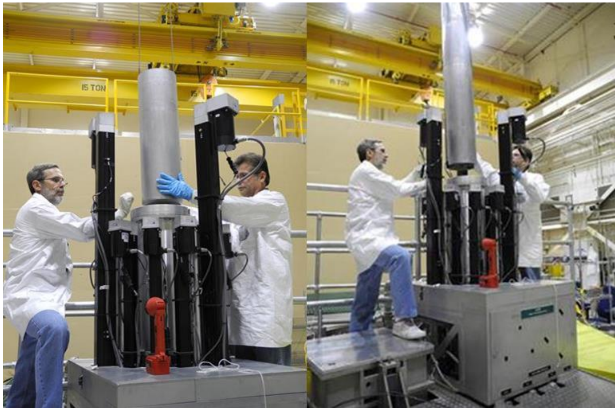
Figure 8. Installing the PLG-1 Bucket (left) and the Shield Plug (right) Into the ACRR Central Cavity.
