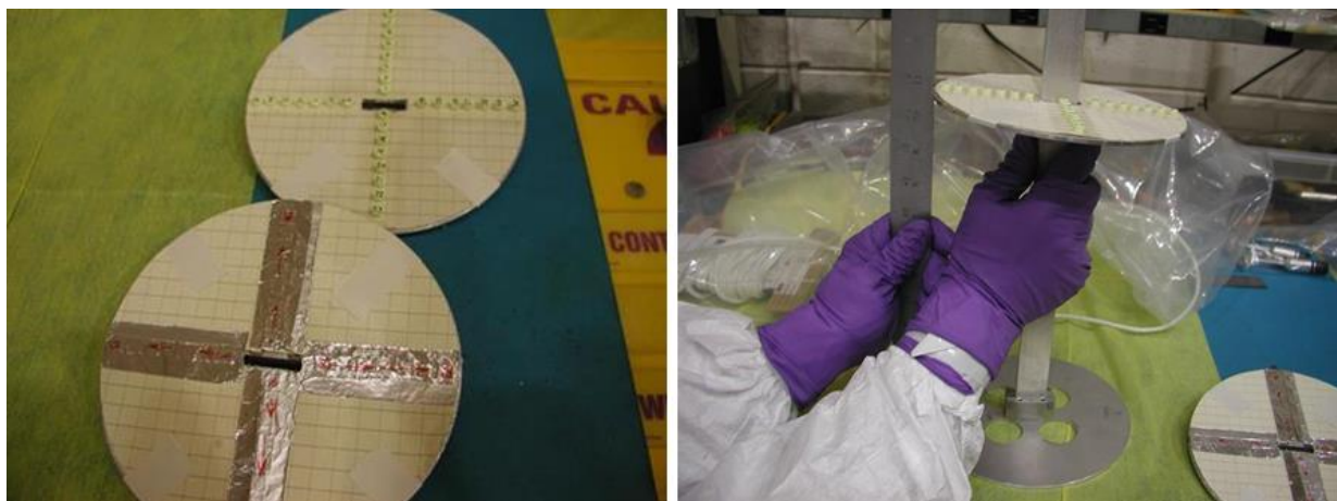
Figure 31. Radial Profile Mapping Fixture for Sulfur Tablets and Gold Foils.
