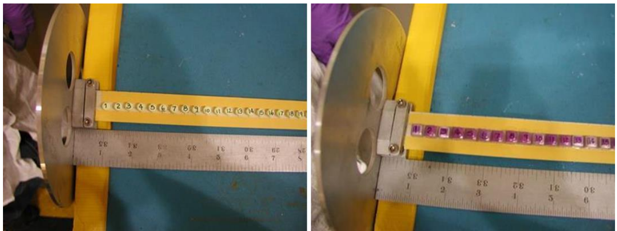
Figure 30. Axial Profile Mapping Fixture for Sulfur Tablets (left) and TLDs (right).
