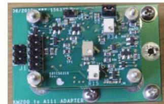
Fig 2c. KM200 as a replacement to the JAB-01 board (top view)
