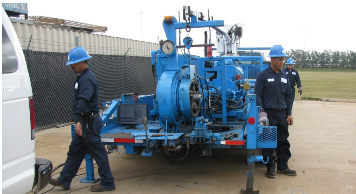
Figure 25. Torque test machine to establish proper makeup torque and to test the tool joint torque strength.
