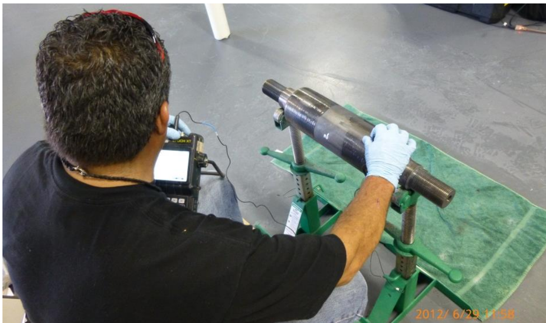
Figure 39. Non-destructive testing of the tool joints used for the FOSS deployment system. The test shown is an Ultra sonic test. Any shallow or deep fractures in the welds show up as reflection anomalies in the ultra-sonic data.
