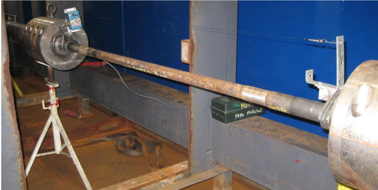
Figure 33. Destructive testing of the drill pipe used for the OpticSeis® deployment system. The steel used in the drill pipe is an S135 steel which is qualified to be used for offshore drill pipe.
