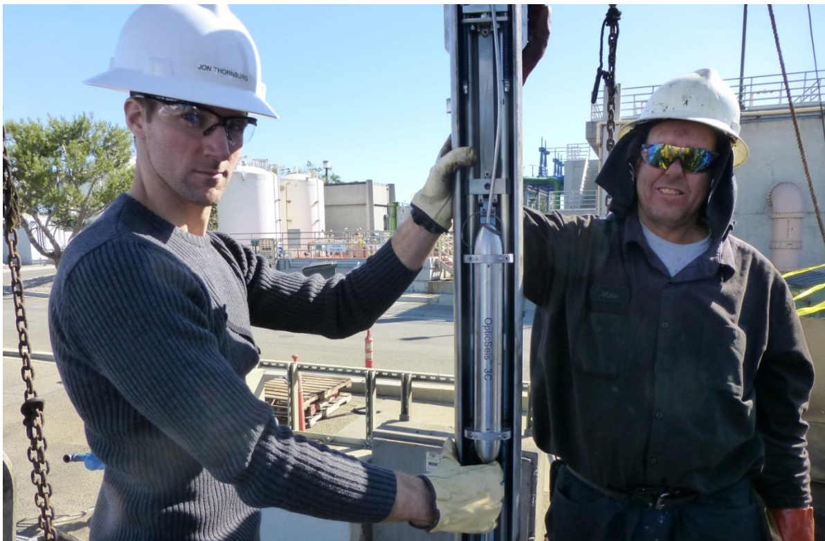
Figure 55. Long Beach, CA. The OpticSeis ® pod placed in the Sensor Pod Housing unit. The Sensor Pod Housing protects the sensor pod during the deployment and also houses the clamping mechanism which securely clamps the sensor pods to the inside of the borehole wall.
