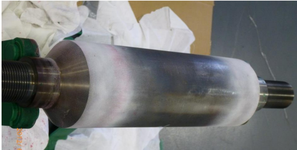
Figure 38. Non-destructive testing of the welded joints used for the FOSS sensor pod housing. The test shown is a penetrant dye test. Any surface fractures in the welds show up as thin red lines.
