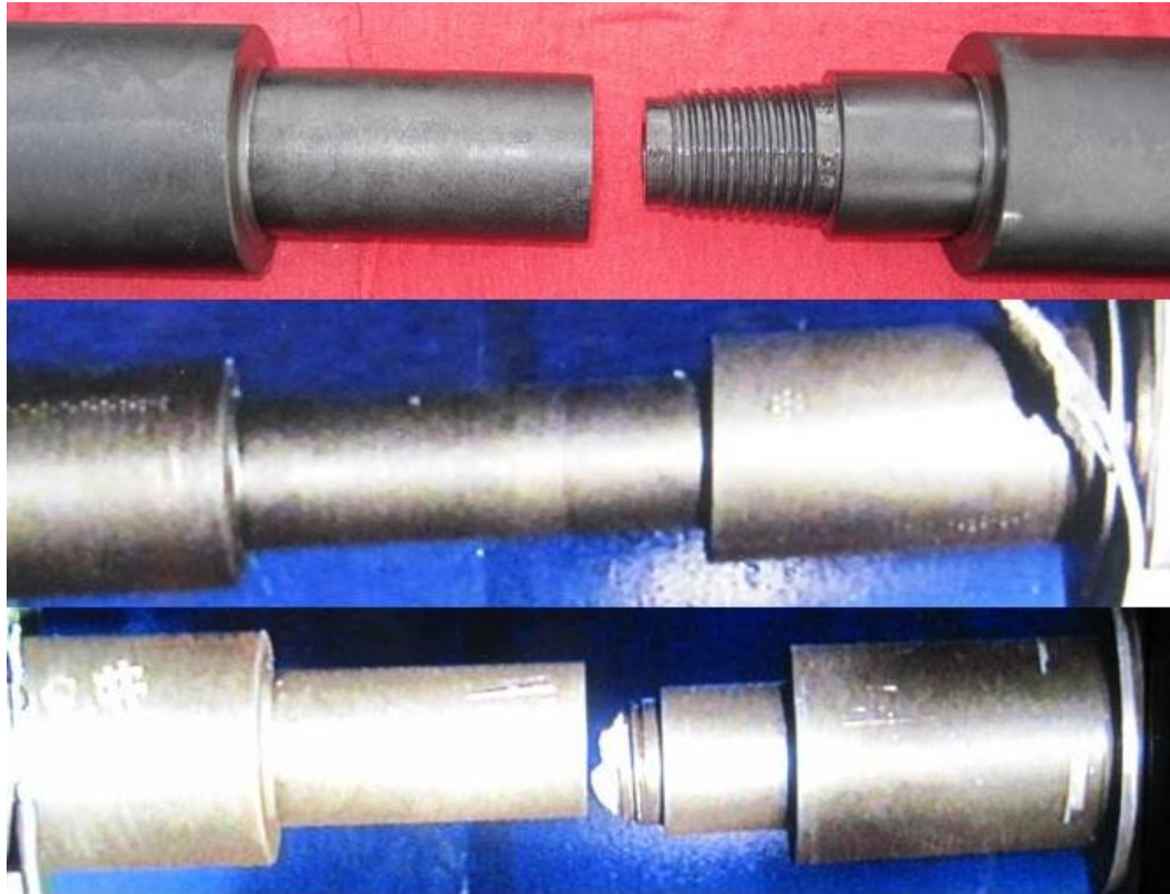
Figure 23. Destructive pull testing of the tool joints used for the FOSS deployment system
