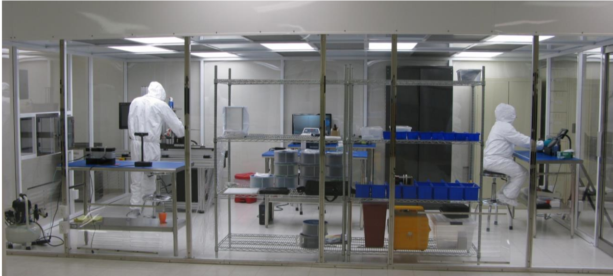
Figure 8. This photo shows the 1,000 rated clean room designed for the manufacturing of the Fiber Optic Seismic Sensors (FOSS) TM . The air in a 1,000 rated clean room is 1,000 times cleaner than the air outside the clean room.
