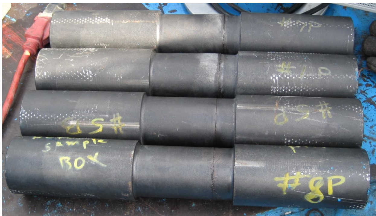
Figure 26. Samples of tool joints after destructive (#7 and #6) and non-destructive (#5 and #8) torque tests.
