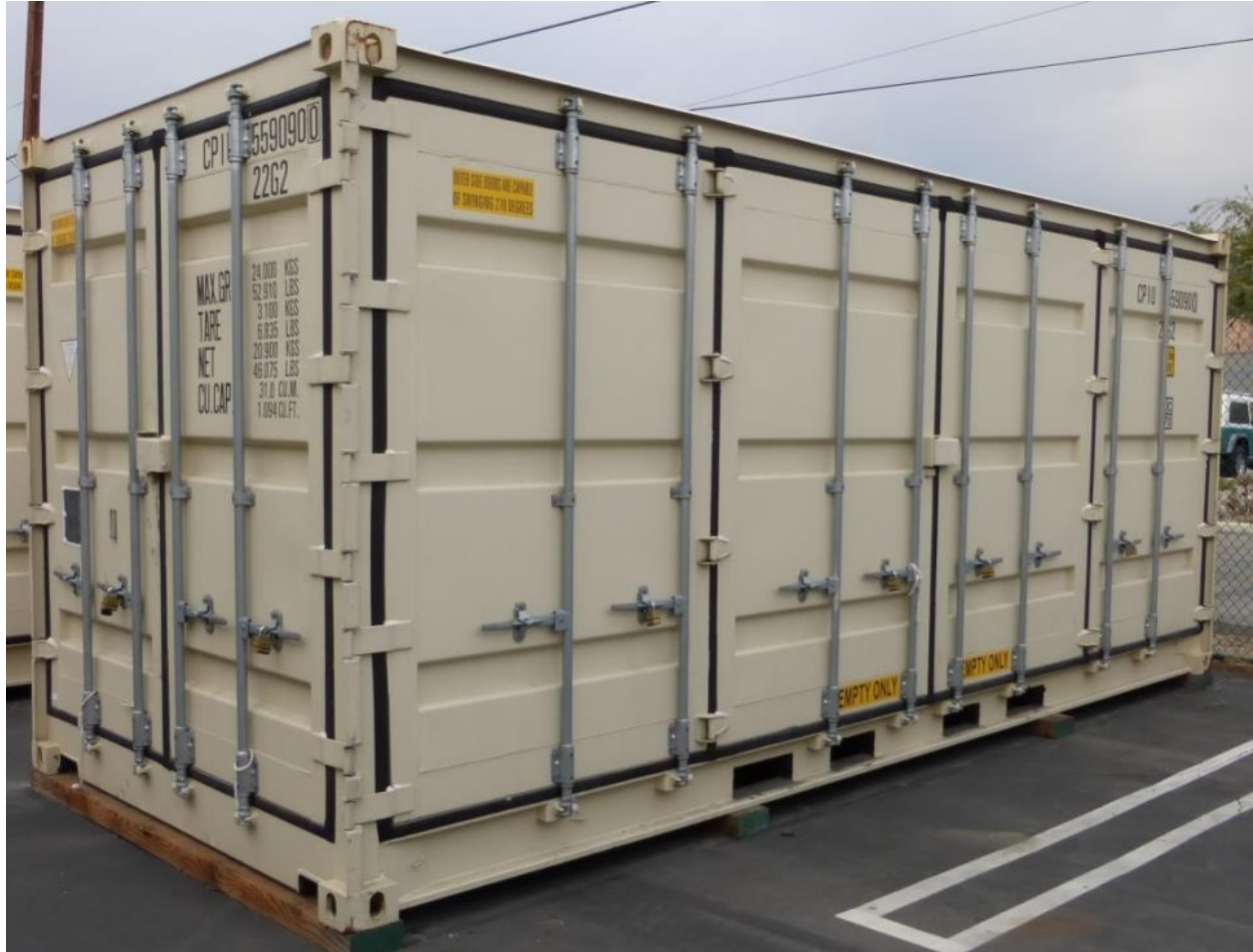
Figure 51. The specialized 20 ft field container that will serve as the doghouse for the redeployable borehole seismic system. The powered spool shown in Figure 50 is designed to fit into the container. There is also room in the container for the interrogator instruments, recording system, observers and data processors.
