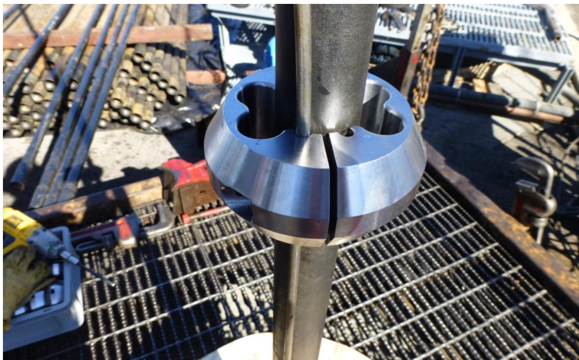
Figure 56. Long Beach, CA. This figure shows the centralizer placed on the small diameter drill pipe. The centralizer is holding and protecting the \frac{1}{4} " steel tubing containing the fibers for the OpticSeis ® sensors. Space has been made for additional cables and \frac{1}{4} " tubes.
