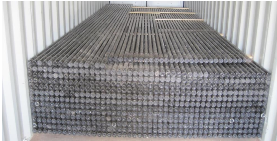
Figure 49. The small diameter drill pipe with an OD 1.660" that is used to deploy the OpticSeis ® system.
