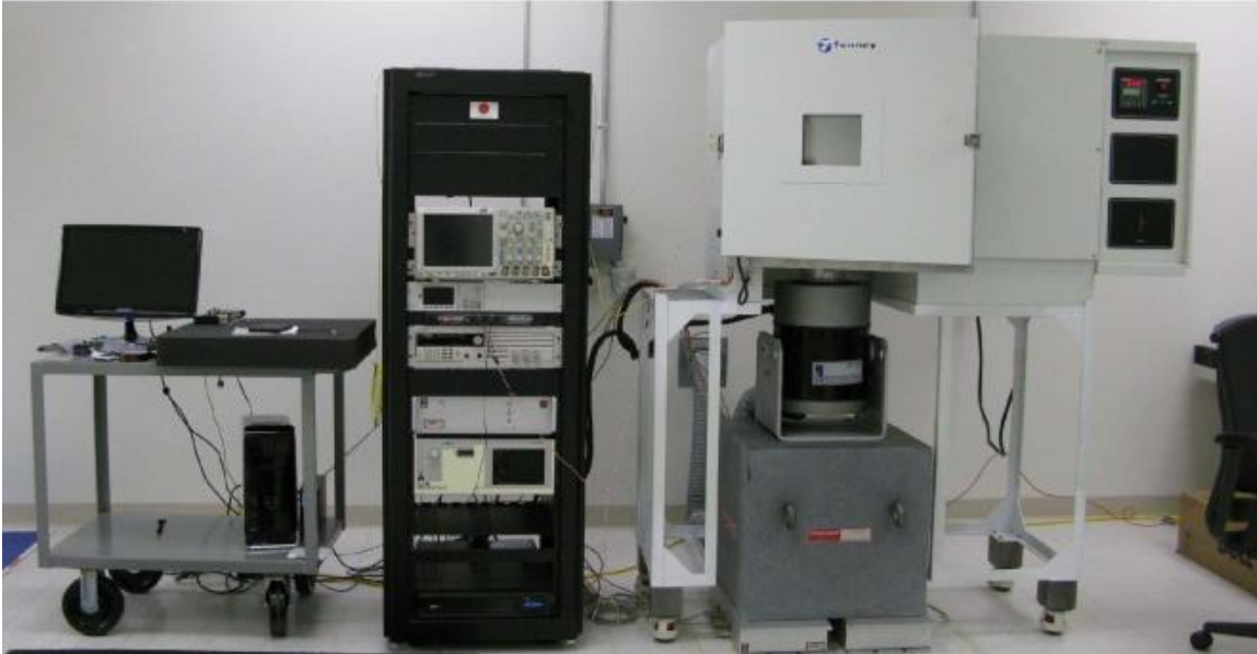
Figure 9. The dynamic test station for the Fiber Optic Seismic Sensors (FOSS) TM . This test station can test the sensor at both low (-65°C) and high (200°C) temperatures at frequencies from 5 Hz to 4,000 Hz.
