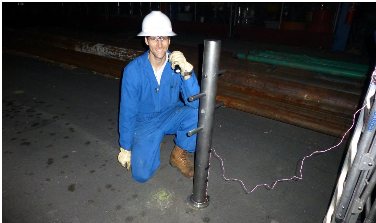
Figure 59. Long Beach, CA. The source used for the Long Beach survey was a 110 lbs. solid steel bar with holes drilled for the handles. The zero time was recorded using a time break accelerometer which is mounted near the bottom of the source.
