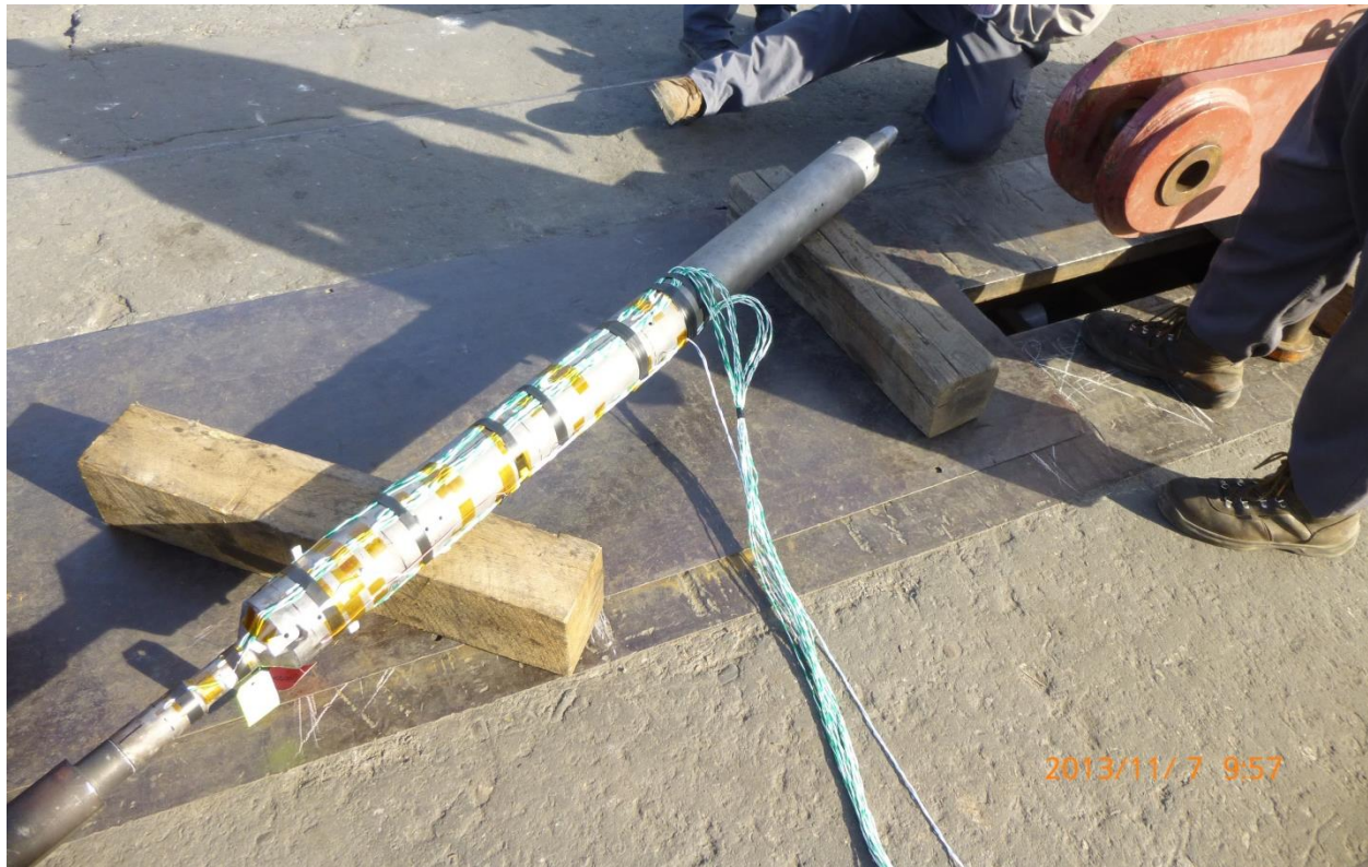
Figure 40. One of four sensor pod housings instrumented with 16 strain gauges in preparation for destructive and non-destructive tests.
