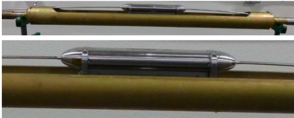
Figure 48a. The Sensor Pod installed into a Sensor Pod Housing. Figure 48b. The 3C Fiber Optic Seismic Sensor (FOSS) ™ packaged into a 16" long and 2" in diameter pod capable of operating at an external pressure of 30,000 psi and an ambient temperature of 320°C (608°F).
