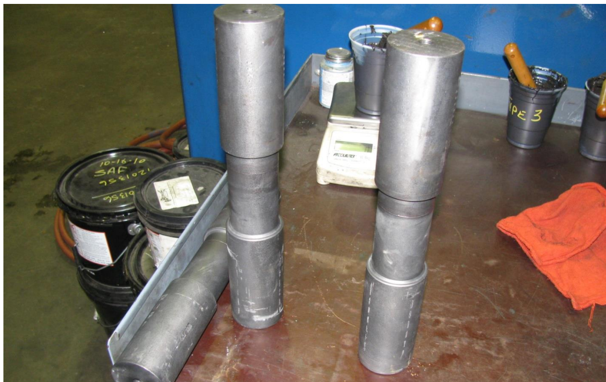
Figure 31. Two samples of Fiber Optic Seismic System tool joint prepared for hydro tests.
