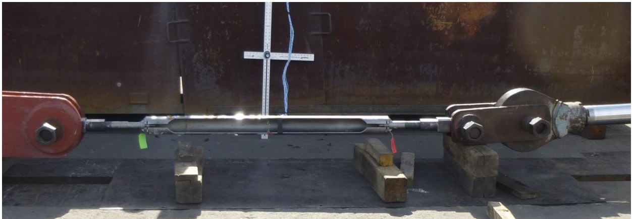
Figure 41. One of four sensor pod housings tested using destructive and non-destructive pull tests.
