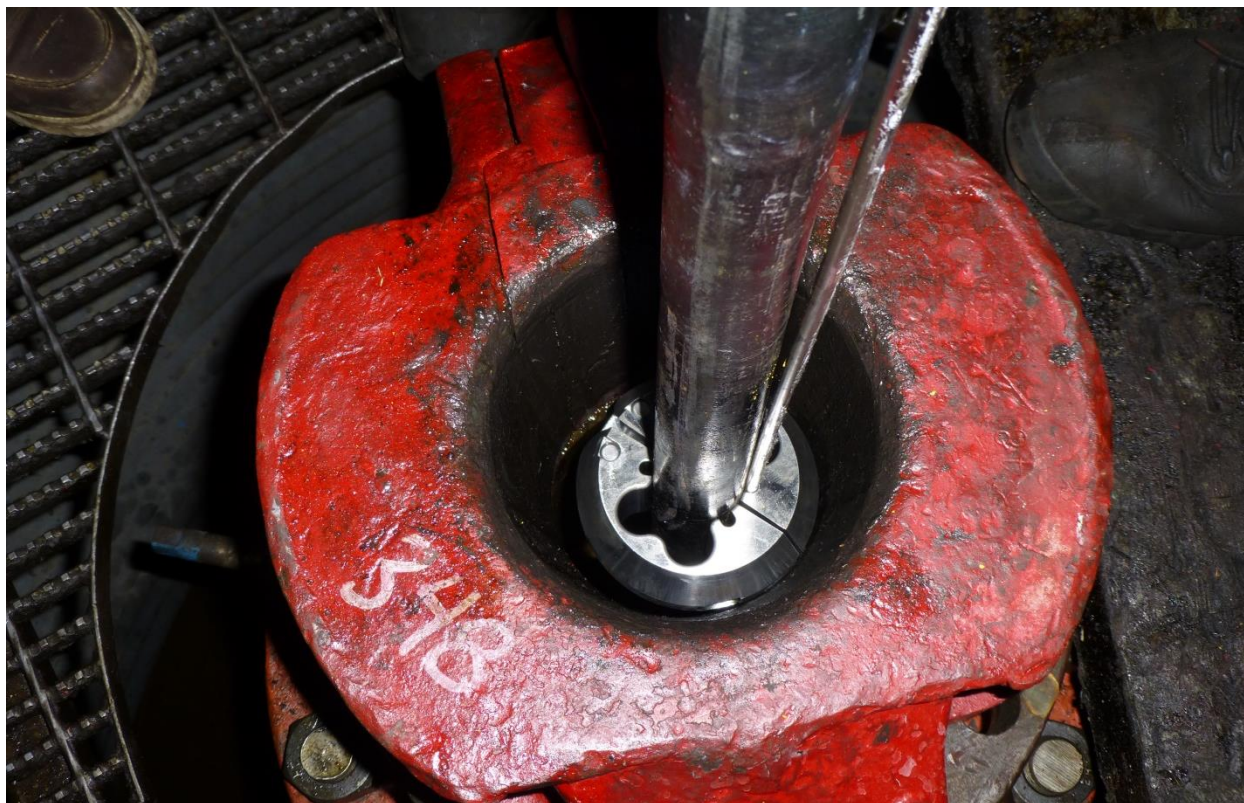
Figure 58. Long Beach, CA. The centralizer is used to protect the 1/4" tubing holding the fiber.
