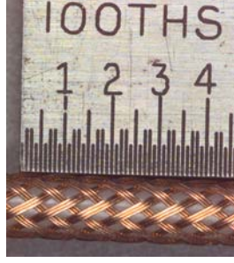
Figure 3. Relatively low ( \approx 60\% ) optical coverage braid illustrating the inherent braid apertures (figure for Remee 1400 cable from [1]).
