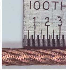
Figure 5. Medium ( \approx 78\% ) optical coverage braid (figure for Belden 9201 cable from [1]).
