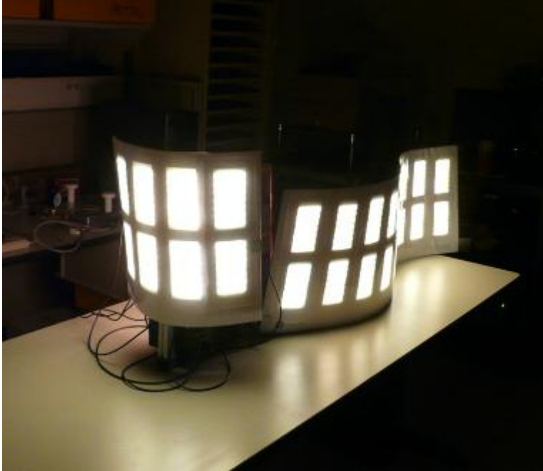
Figure 2: The large area, 900 lumen, thin and flexible luminaire delivered by this project
