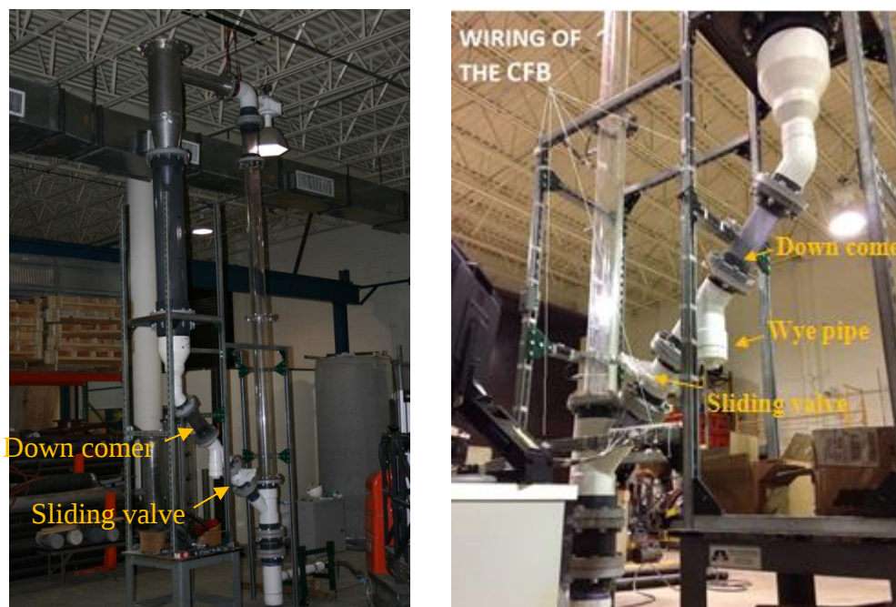
Figure 8. Completed solid feeding mechanism in the circulating fluidized bed set-up at FIU
