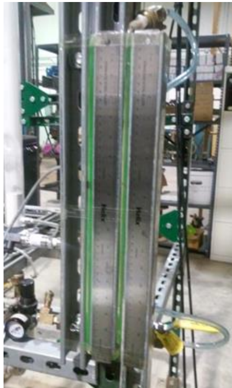
Figure 20. Monometer that was fabricated in FIU ARC laboratory for pressure measurements.
