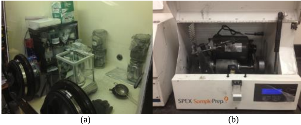
Figure 6. a) The Labconco glove box, b) A SPEX 8000M Mixer/Mill available at the Advanced Materials Laboratory, University of Idaho.
