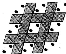
Figure 1. Structure of the titanium-based spinel  $\text{Li}_4\text{Ti}_5\text{O}_{12}$ . Black spheres represent lithium cations; gray polyhedra represent  $[\text{Ti}(\text{Li})\text{O}_6]$  octahedra.
