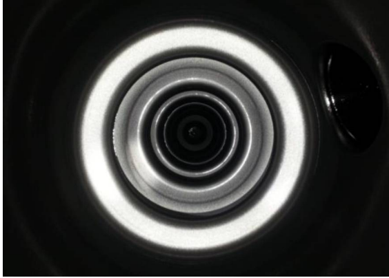
Figure 6: 5-cell cavity RF surface after BCP.
