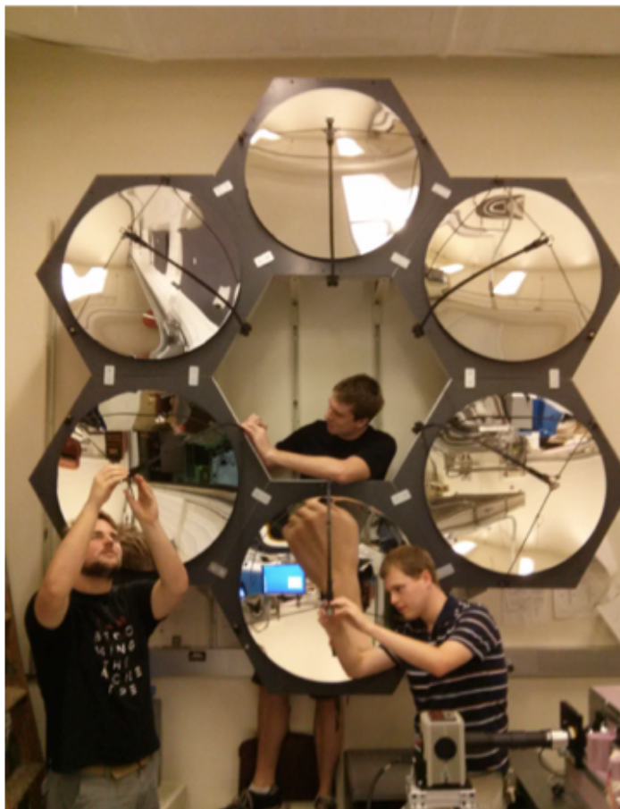
Figure 5: Projector prototype. A total of 6 mirrors, each attached to an aluminum hexagon structure with attached collimator and holographic diffuser system.
