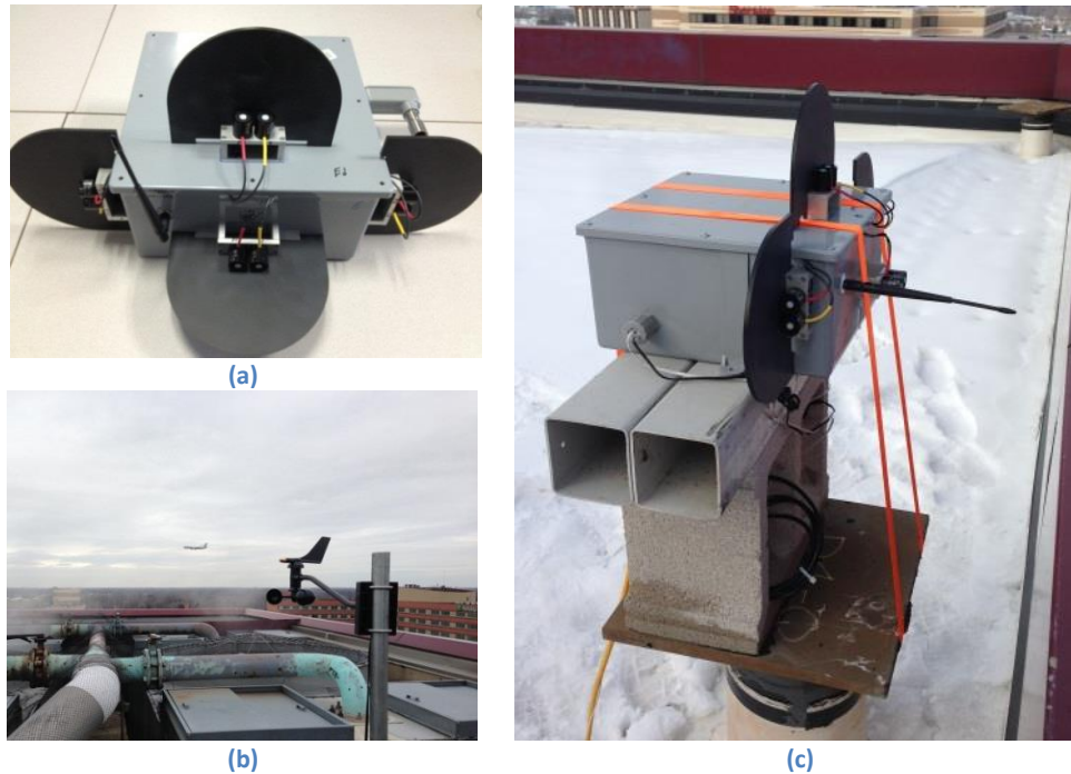
Figure 33 (a) exterior sensor enclosure hosting photosensors, pyranometers and temperature sensors; (b) anemometer; (c) exterior sensor enclosure mounted in place.
