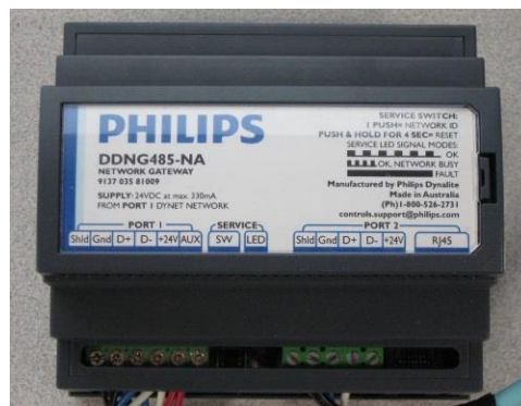
Figure 35 DDNG485 network communication gateway.
