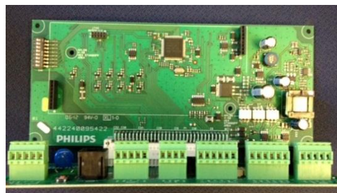
Figure 37 ECoMIC controller board (ECB).
