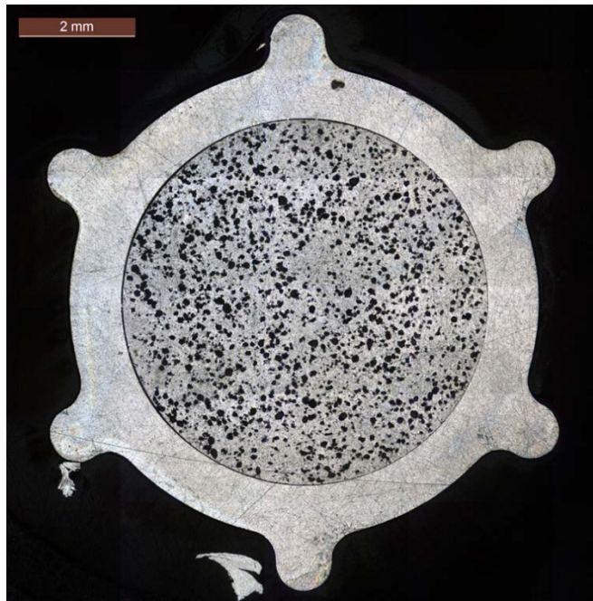
Figure 5. Cross section of partial length target showing the pellet clad gap after irradiation (P-94, pellet #4, mount 6395).
