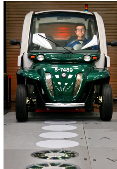
Fig. 4. The ORNL NEV ready to receive WPT dynamically.
