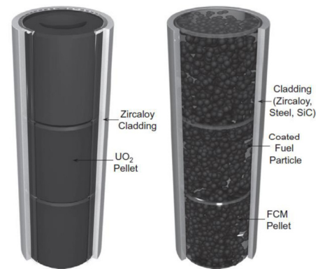
Fig. 2. Comparison of standard \text{UO}_2 /Zircaloy fuel (left) and an FCM fuel pin (right) [3].
